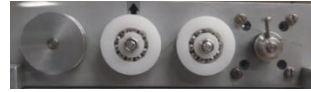
Figure 22 Pulley system, from left to right: distance encoder, load cell, support pulley, stepper motor
