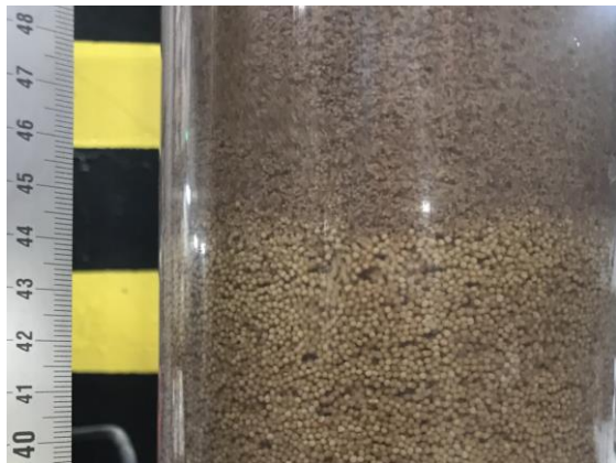
Figure 122 Two-fractions mixture: crushed calcite grains 0.50-0.63 mm at the top and calcite pellets 1.25-1.40 mm at the bottom
