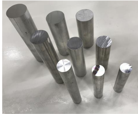
Figure 117 Aluminium cylindrical objects, ( L_{co} = 100, 120, 160 mm · D_{co} = 20, 30, 40 mm), \rho_p = 2,701 kg/m 3
