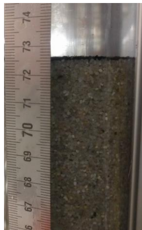
Figure 95b Fixed bed setting after t=5 [min] ETSW
