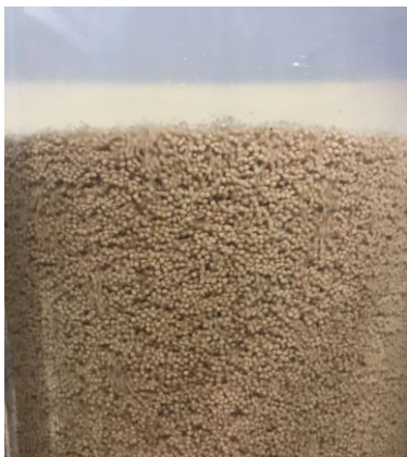
Figure 121 Single fraction experiment 0.9-1.0 mm calcite pellets
