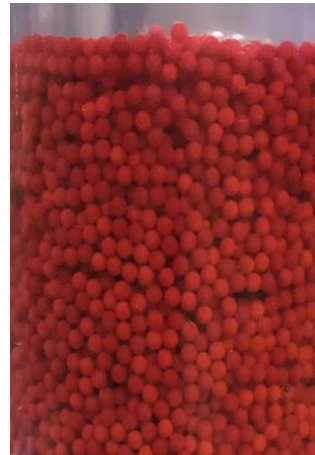
Figure 57 Fluidised glass beads in water just above incipient fluidisation (2.5 mm 22 °C, 39 mm/s)
