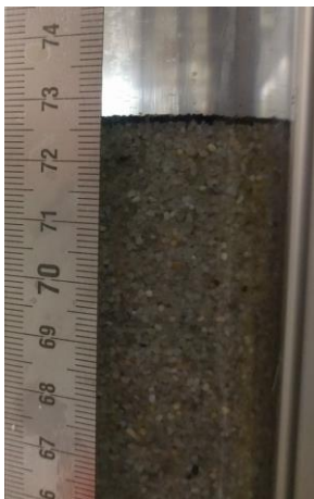
Figure 95a Initial fixed bed
