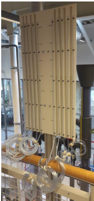
Figure 17 Hydrostatic measurement board with longitudinal taps
