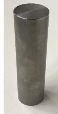
Figure 118 Titanium cylindrical object, ( L_{co} = 130 , · D_{co} = 35 mm), \rho_p = 4,464 kg/m 3
