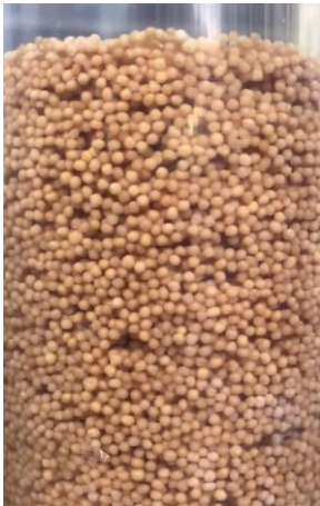
Figure 55 Fluidised calcite pellets in water at normal fluidisation: voids are clearly visible (1.4-1.7 mm 20 °C, 22 mm/s)
