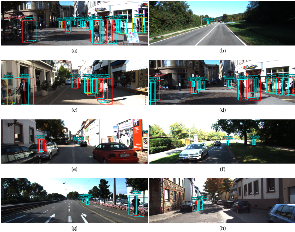
Figure 5.3: Qualitative results for the proposed model on the KITTI validation set. The model can estimate the 3D location of people with different orientations and poses. (a) - (d): examples with good performance on crowded scenes, far away objects, occluded and truncated objects. (e) - (h): failure cases with missed detections, false positives and confusions with cyclists. Ground truth: red. Predictions: cyan. Numbers on top of boxes: detector objectness, IoU.
