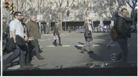
(b) Truncation of person on left image border and hood of the ego-vehicle; occlusion by other pedestrians.
