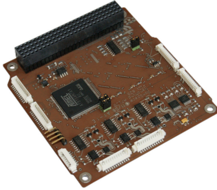
Figure 2.2: Existing OBC for Nano satellites [1]
