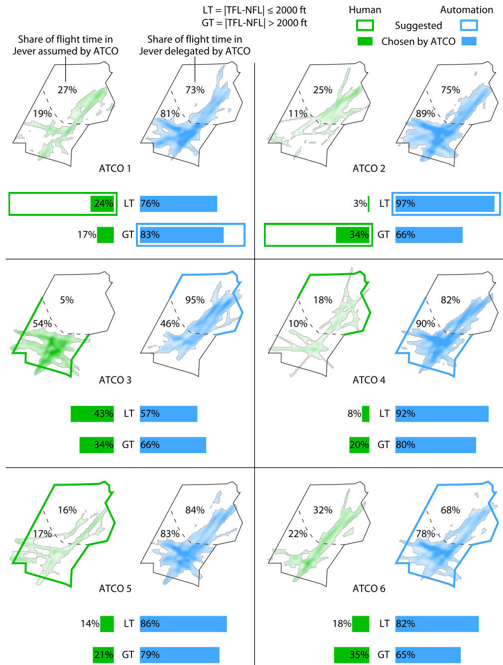
Figure 16. Flight density maps and share of flight time as allocated by the ATCOs, split per agent; the colored outlines indicate the suggested allocation from Figure 11, i.e., the absolute required flight level change |\Delta FL| between sector entry (NFL) and transfer to the next sector (TFL) for ATCOs 1 and 2, entry sector for ATCOs 3 and 4, and all manual or automated for ATCOs 5 and 6.
