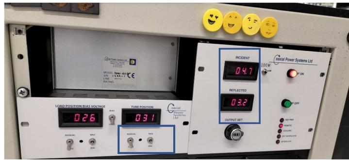
Figure 2.14: Tuning of reflected power.
