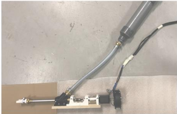
Motorized extruder connected to the clay cartridge
