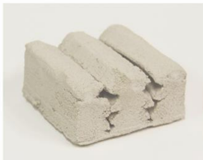
Triangular, parallel extrusion, p=1369 \text{ kg/m}^3
