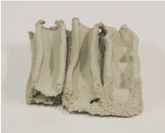
Fig.: 53, U-5 Nozzle, straight, parallel extrusion, five layers on top of each other. Collapsing layers
