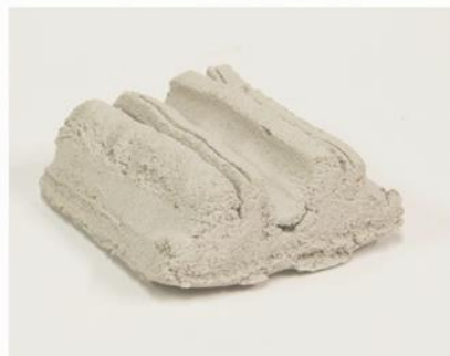
U-shaped Nr.3, parallel extrusion, p=1184 \text{ kg/m}^3
