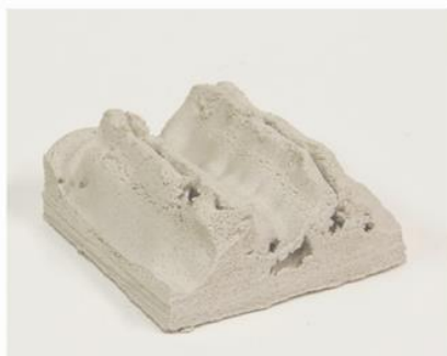
U-shaped Nr.5, parallel extrusion, p=997 \text{ kg/m}^3
