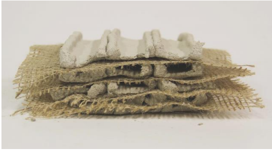
Fig.: 65, U-5 Nozzle, parallel extrusion with jute mesh in between each layer. height: 5 layers, each 12mm
