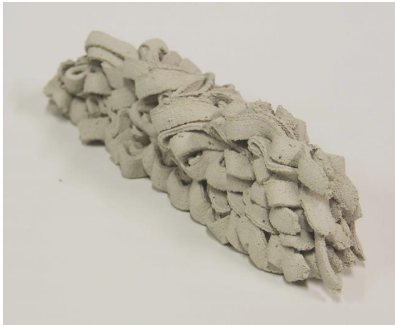
Fig.: 62, “Tagliatelle” Nozzle- same principle as the “Spaghetti” nozzle
