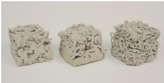
Fig.: 60, Spaghetti nozzle. The thin nozzle openings create small clay strings. These strings enclose air. Right: r=2\text{mm} , Middle: r=3\text{mm} , Right: r=4\text{mm}
