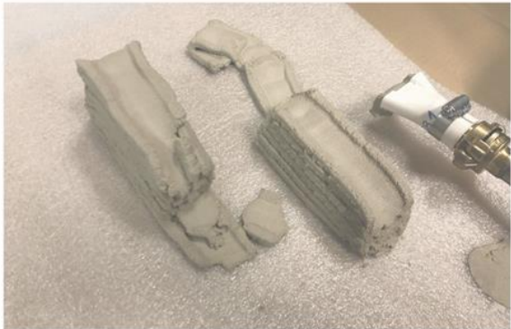
The motorized extruder allows to extrud mixture with less water content.
