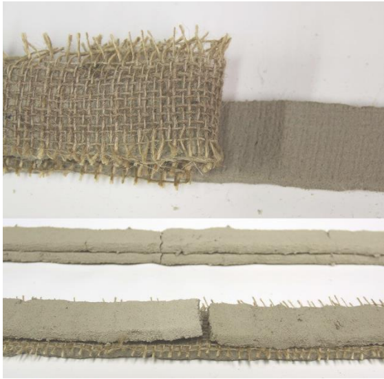
Fig.: 69, Top: bonding between mesh and clay mixture Bottom: Two 90cm long, stacked rectangular (12x40mm) extrusions. Back: Without fibre reinforcement, front: one fibre mesh between the two layers
