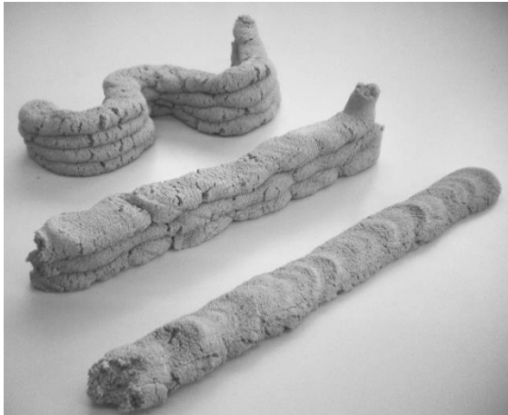
Fig.: 43, Mixture 6 perpendicular extruded on the print surface. single layer, stacked layer linear. stacked layer S-Shape
