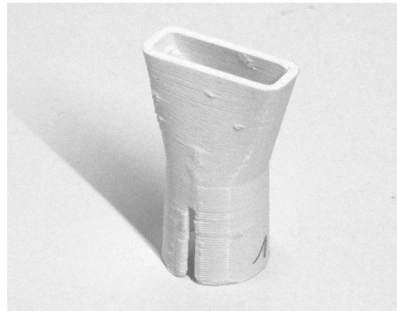
Fig.: 28, Rectangular Nozzle, h:12mm, w:40mm, fillet r=2mm
