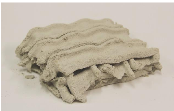
Fig.: 56, U-5 Nozzle, cross extrusion, five layers on top of each other. The direction gets changed every other layer- lower risk of collapsing layers
