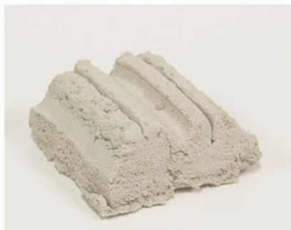
U-shaped Nr.2, parallel extrusion, p=1197 \text{ kg/m}^3
