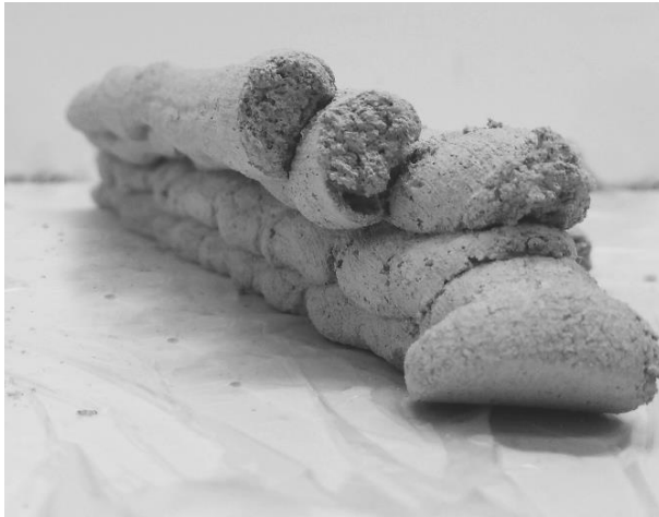
Fig.: 45, stacked layers with laid down extrusion and 60+° overhang
