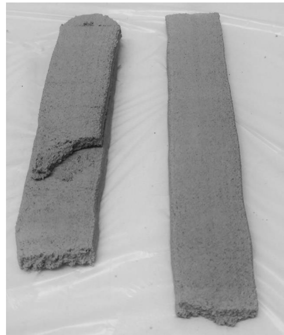
Fig.: 47, Straight rectangular Nozzle extrusion. h: 12mm, w: 40mm, edge fillet r=2\text{mm} , A=430\text{mm}^2
