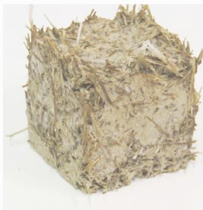
Solid "loose" straw clay cube, p=600 \text{ kg/m}^3
