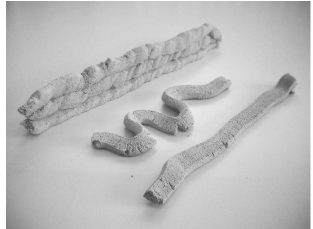
Fig.: 42, rectangular nozzle, linear and S-shape single layer, stacked layer extrusion
