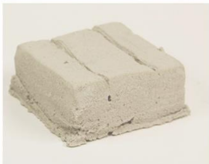
Rectangular, parallel extrusion, p=1747 \text{ kg/m}^3
