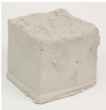
Solid cast Cube, p=1629 \text{ kg/m}^3
