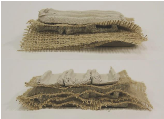
Fig.: 66, U-5 Nozzle, crossed extrusion with jute mesh in between each layer. height: 5 layers, each 12mm
