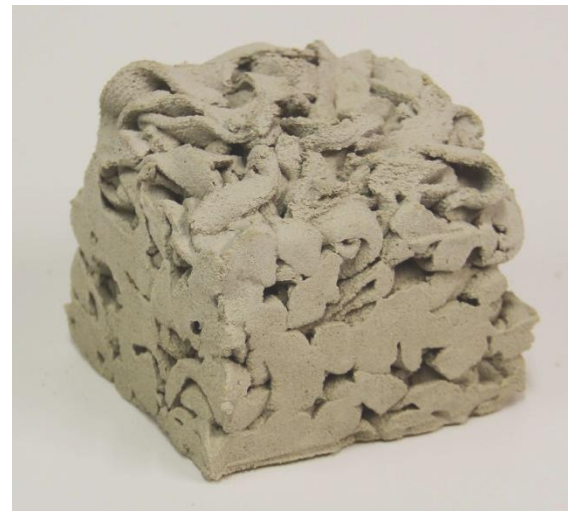
Fig.: 61, “Tagliatelle” Nozzle- same principle as the “Spaghetti” nozzle. 10x rectangular openings of 3 \times 12\text{mm}
