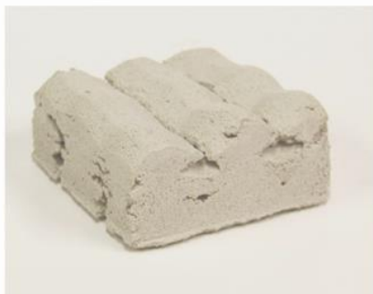
Triangular, crossed extrusion, p=1362 \text{ kg/m}^3
