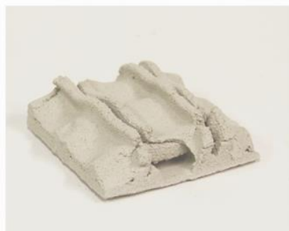
U-shaped Nr.2, crossed extrusion, p=773 \text{ kg/m}^3
