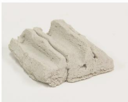
U-shaped Nr.4, parallel extrusion, p=1073 \text{ kg/m}^3
