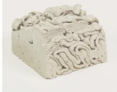
S-Shaped waved extrusion, p=1441 \text{ kg/m}^3
