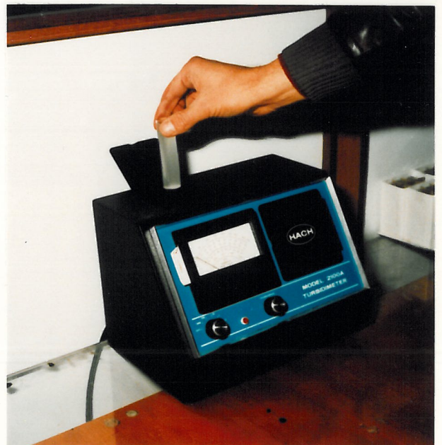
no 4. Turbidity meter
