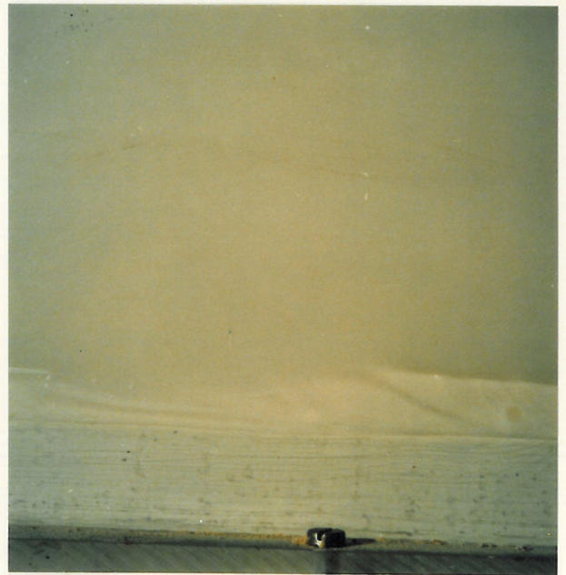
no 8. Vortex motion above consolidated bed (T3-4)
