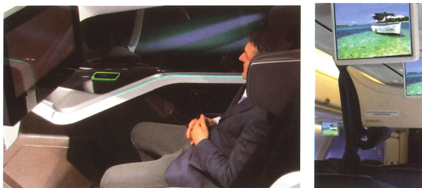
Figure 8. A screen in front of a person (left) should have different back rest angles than a screen mounted to the ceiling (right).
