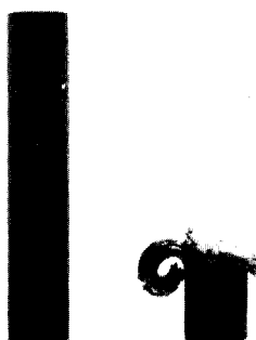
Figure 4.32 Recovered steel rod after impact of an armour of 8.1 mm alumina backed by 4.0 mm aluminium at a velocity above the v_{50} (829 m/s).
