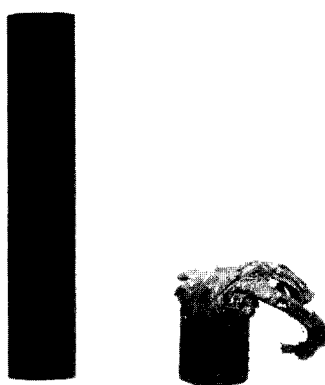
Figure 4.15 Recovered steel rod after impact of an armour of 8.1 mm alumina backed by two 3.0 mm thick layers aluminium at a velocity below the v_{50} (819 m/s).
