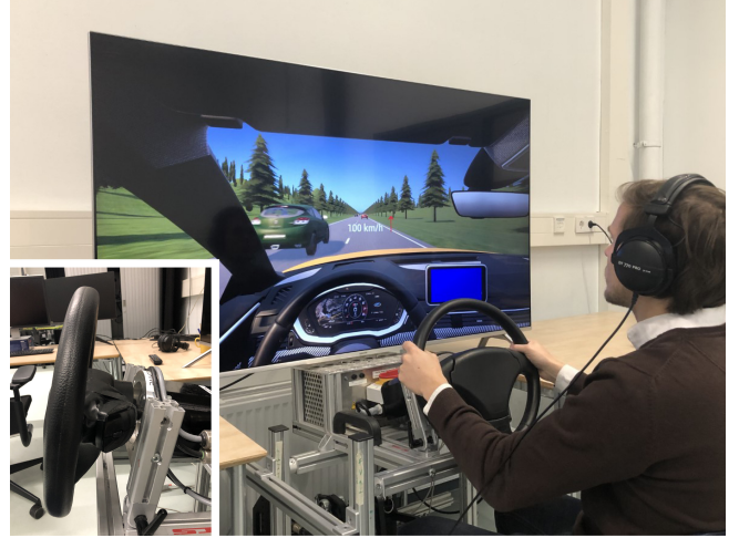
Fig. 1. The hardware setup and virtual simulator environment during the experiment. The blue dashboard display shows the communication to the driver about the steering response in use. Left bottom corner shows the attached mouse for driver-initiated steering.
