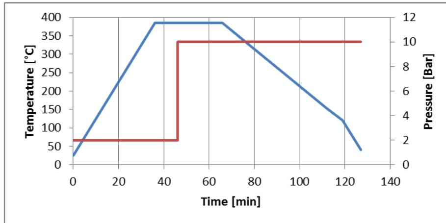
Figure 2. Press cycle. Blue line indicates temperature and red line indicates pressure.
