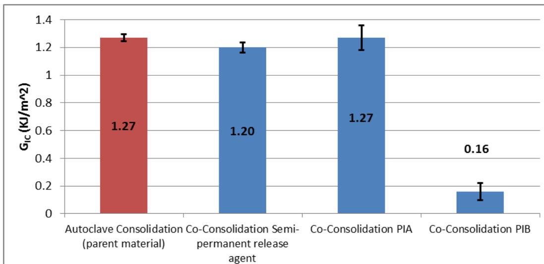
Figure 6. Delamination fracture toughness of different samples.
