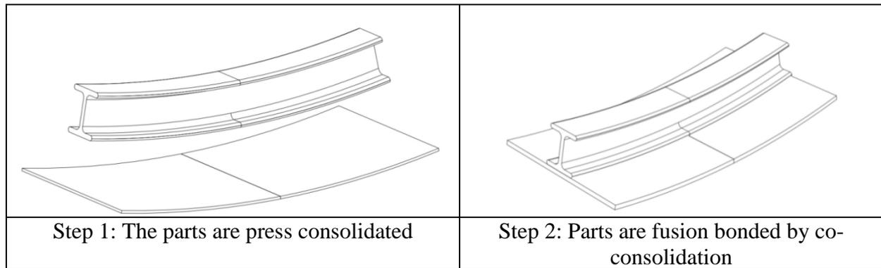
Figure 1. Schematic of the two-step consolidation process (Co-consolidation)
