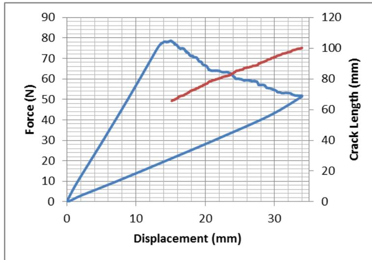
Figure 5. Blue line indicates force vs. displacement curve, and red line indicates crack length vs. displacement.
