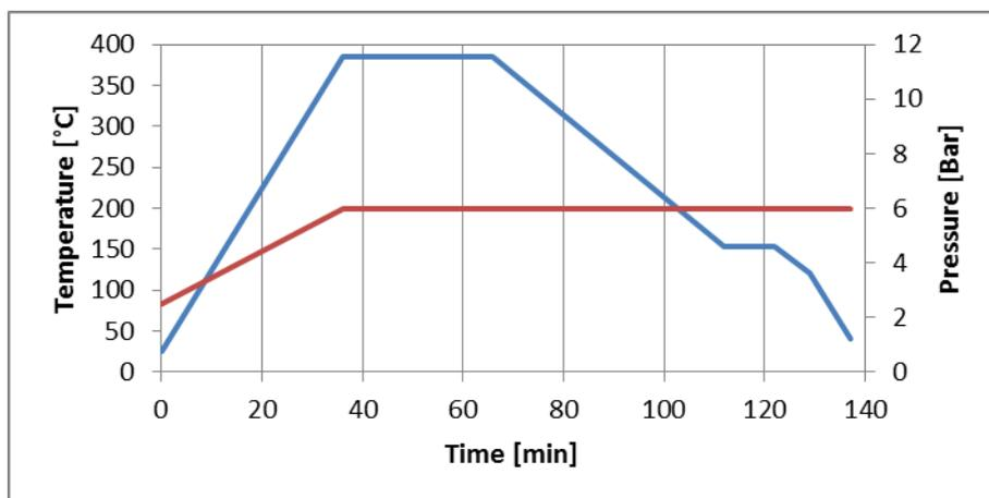
Figure 4. Autoclave cycle. Blue line indicate temperature and red line pressure.
