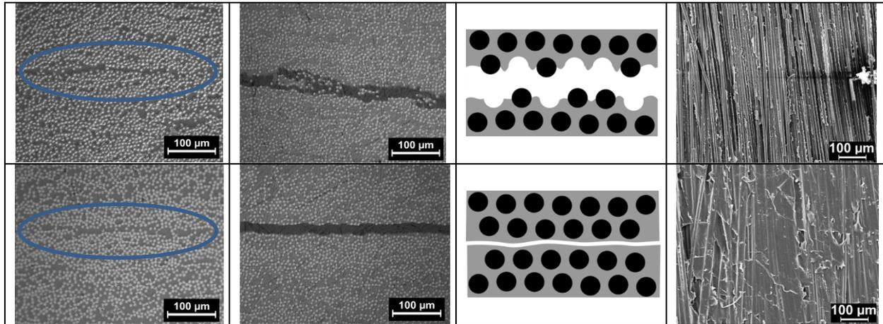
Figure 7. From left to right, cross section micrographs before testing (the blue circle indicates the interfaces), cross section after testing, scheme of the failure, and SEM micrograph of the fracture surface. From top to bottom, one step press consolidation of 24 layers, and co-consolidation with Polyimide B release media.
