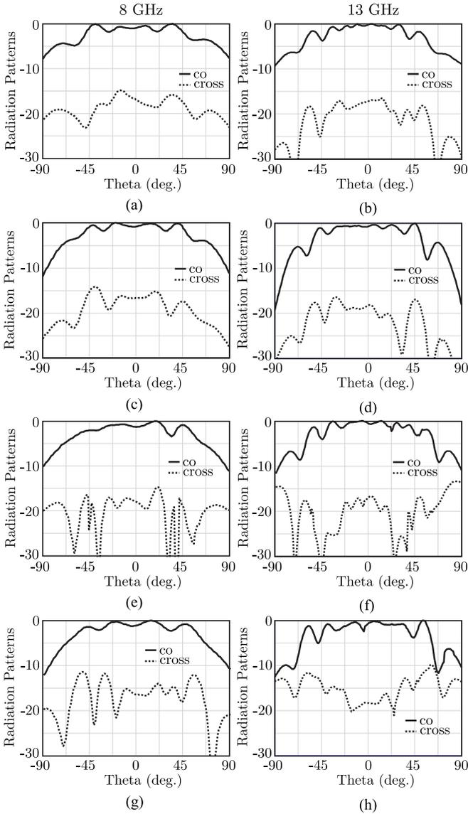
Fig. 10. Measured normalized co-pol and X-pol active element patterns of a central element of the array at 8 GHz and 13 GHz: (a), (b)  $E$ -plane; (c), (d)  $H$ -plane; (e), (f)  $D$ -plane  $\phi = -45^\circ$ ; (g), (h)  $D$ -plane  $\phi = 45^\circ$ .
