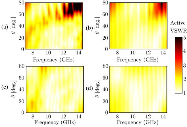
Fig. 8. Measured active VSWR of a central element of the array as a function of frequency and scanning angle in the (a)  $H$ -plane without amplitude taper, (b)  $H$ -plane with amplitude taper, (c)  $E$ -plane without amplitude taper, (d)  $E$ -plane with amplitude taper.
