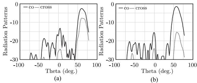
Fig. 13. Measured co-polar and cross-polar radiation patterns for scanning to 60 degrees in the  $D$ -plane: (a)  $\phi = 45^\circ$ ,  $\theta = 60^\circ$  (b)  $\phi = -45^\circ$ ,  $\theta = 60^\circ$ .
