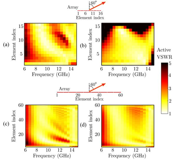
Fig. 5. Active VSWR as a function of frequency and element index: (a), (b)  $16 \times \infty$  elements without and with amplitude taper, respectively; (c), (d)  $60 \times \infty$  elements without and with amplitude taper, respectively; scanning to  $60^\circ$  in the  $H$ -plane is considered.
