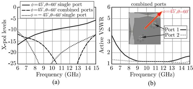
Fig. 4. (a) X-pol levels for scanning in the diagonal planes to  $\theta = 60^\circ$ :  $\phi = 45^\circ$  with single port excitation (continuous line),  $\phi = 45^\circ$  with the two ports excited with proper weights to cancel the X-pol at 12 GHz (dashed line) and  $\phi = -45^\circ$  (dotted line); (b) active VSWR for the two ports when combined to cancel the X-pol for  $\phi = 45^\circ$  and  $\theta = 60^\circ$ .
