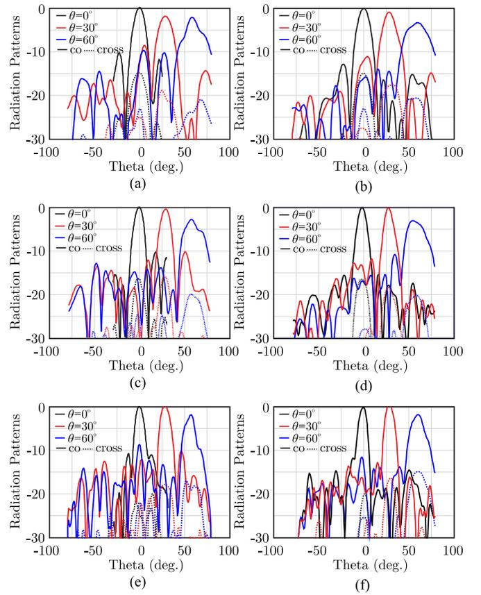
Fig. 12. Measured co-polar and cross-polar radiation patterns for scanning to  $0^\circ$ ,  $30^\circ$  and  $60^\circ$ : (a)  $H$ - and (b)  $E$ -planes at 8.4 GHz, (c)  $H$ - and (d)  $E$ -planes at 11 GHz, (e)  $H$ - and (f)  $E$ -planes at 14.5 GHz.
