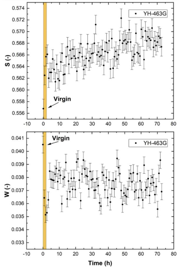
Fig. 3. Time-dependence of the Doppler  $S$ - and  $W$ -parameter collected at a positron implantation energy of 5 keV. The orange-shaded area denotes the time interval of 2 h of *in situ* UV optical illumination of the 330 nm  $YO_xH_y$  sample, after which the LED ( $\lambda = 385$  nm) is turned off and the sample bleaches in dark conditions.
