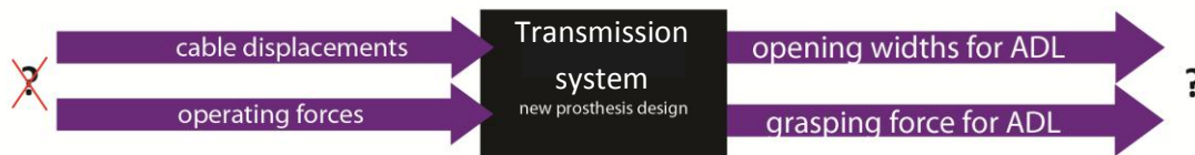
Figure 14. Black box of new prosthesis design. The input is being investigated: operating forces and cable displacements. When also the output is known (opening widths and grasping forces for ADL) it is possible to design the transmission system for shoulder controlled prosthesis with improved cable control.
