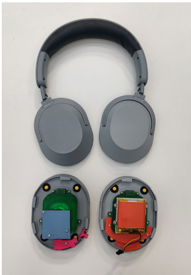
Figure 47. The orientation of the headphones for disassembly is the same as the headphone orientation in the book. The use of different colours creates visual clusters, guiding the user..
