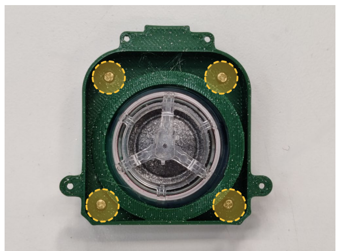
Figure 29. 'Hidden' screws on the underside of the driver housing.
