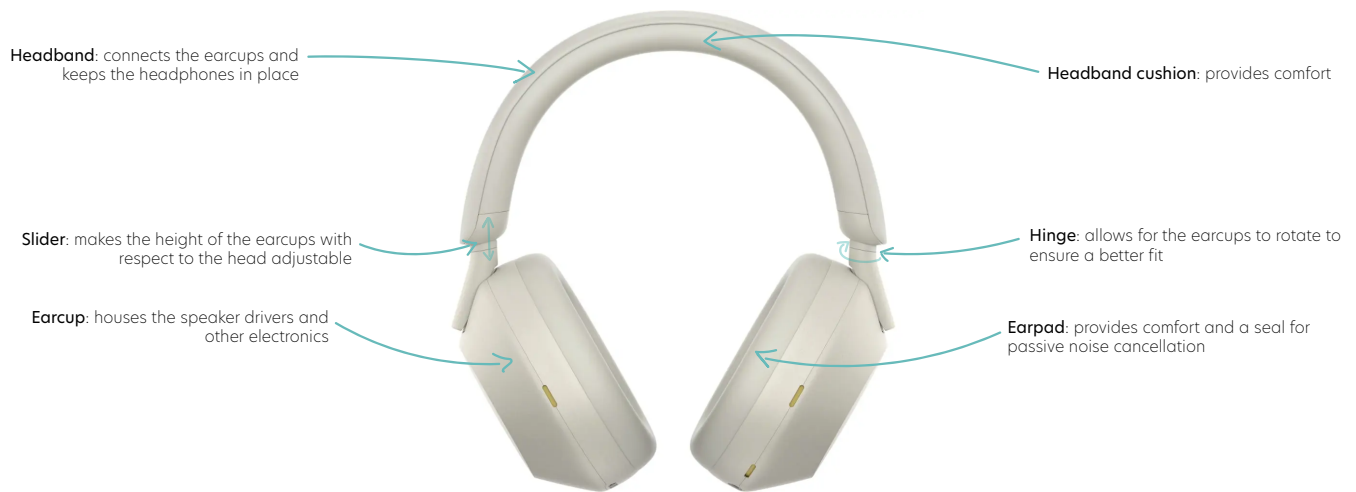
Figure 1. Headphone architecture: structural components (Sony Group, n.d.-d).
