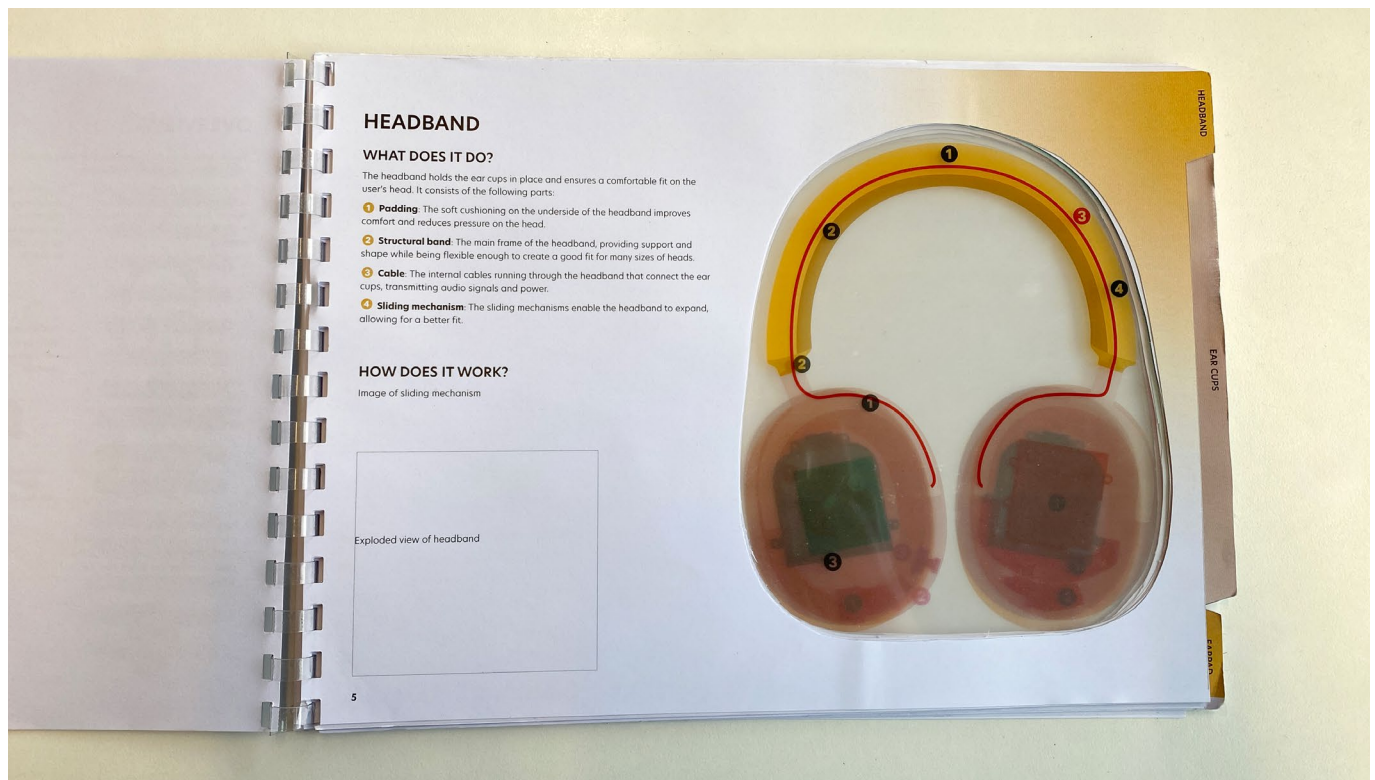
Figure 46. The transparent pages in the book show the headphones in the correct orientation for disassembly. The use of different colours stops the components from blending together.
