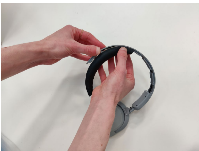
Figure 38. The headband padding can easily be slid on and off.
