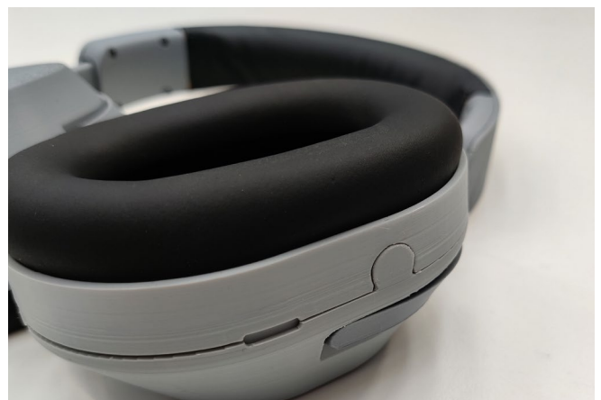
Figure 48. Visible snap fits keep the two halves of the earcup housing together.
