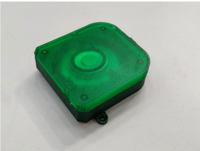
Figure 31. The audio module with its transparent housing.
