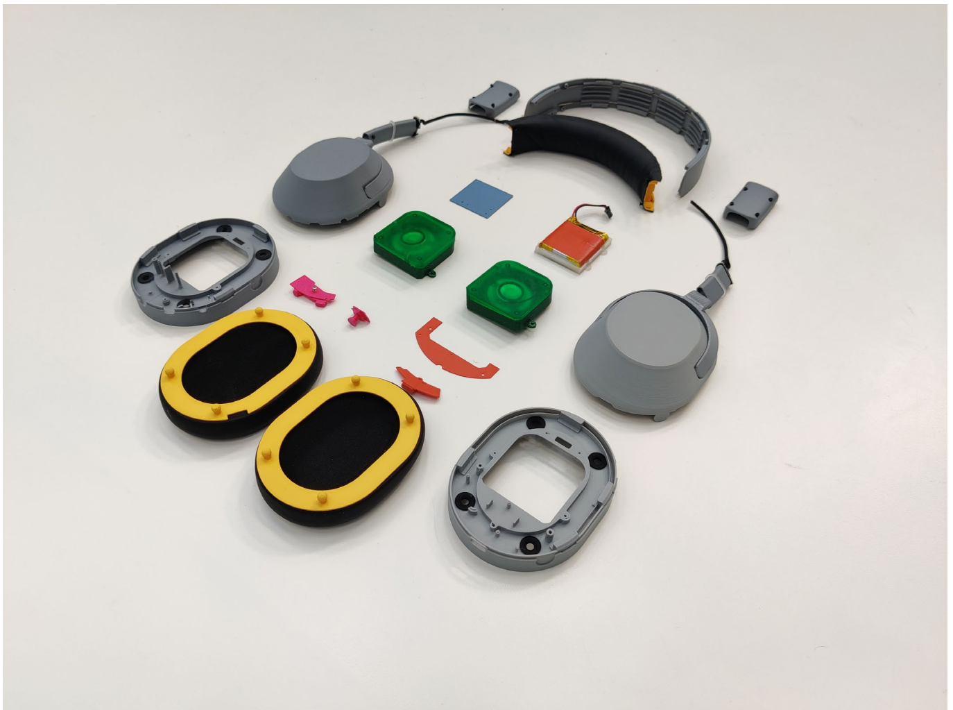
Figure 55. The headphone separated into all its individually replaceable parts and modules .
