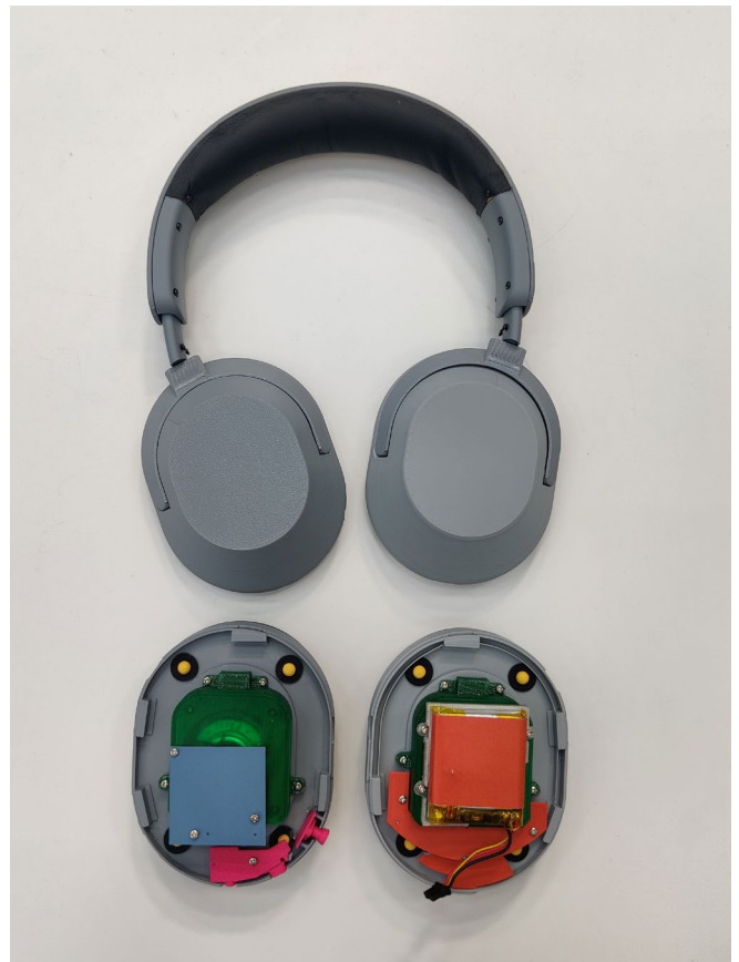
Figure 27. Prototype of the headphones fully assembled (left), and with the shell removed, showing the components inside the earcup (right).
