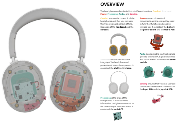
Figure 52. Colour-coding by function in the book makes components visually distinct from each other.
