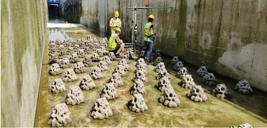
Fig. 2. Deployment of more than 100 artificial reef structures on the reef platform (see [3] for a description of the reef restoration runs).
