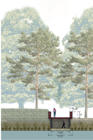
Fig. 8.43: Section detail bridge
