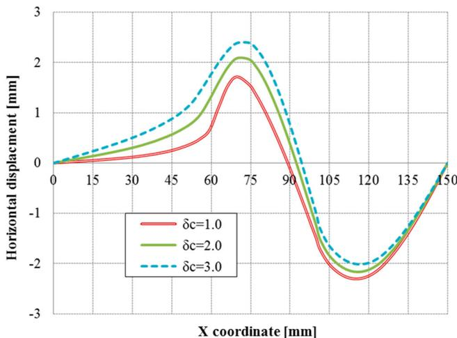
Figure 13. Membrane horizontal displacements ( $G = 4.0$  N/mm,  $\delta_c = 1.0\text{--}3.0$  mm).
