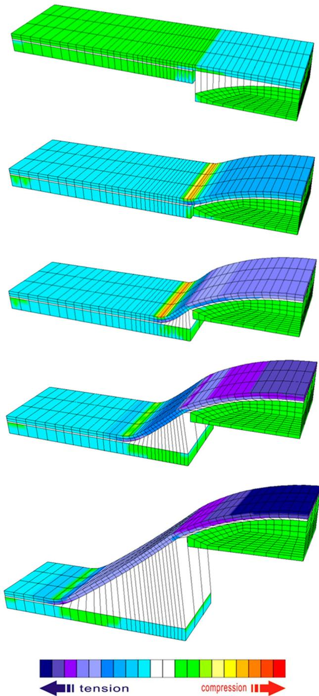
**Figure 18.** Evaluation of horizontal stress of MAT test, piston vertical displacement: 0, 10, 30, 50, 80 mm.
