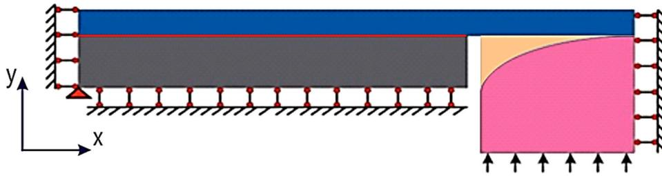
Figure 4. Boundary conditions for MAT FE simulations.
