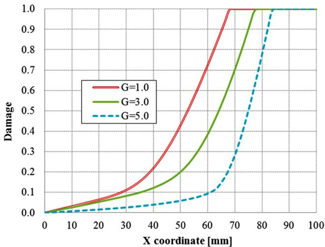
Figure 8. Interface damage ( $G = 1.0\text{--}5.0$  N/mm,  $\delta_c = 2.0$  mm).
