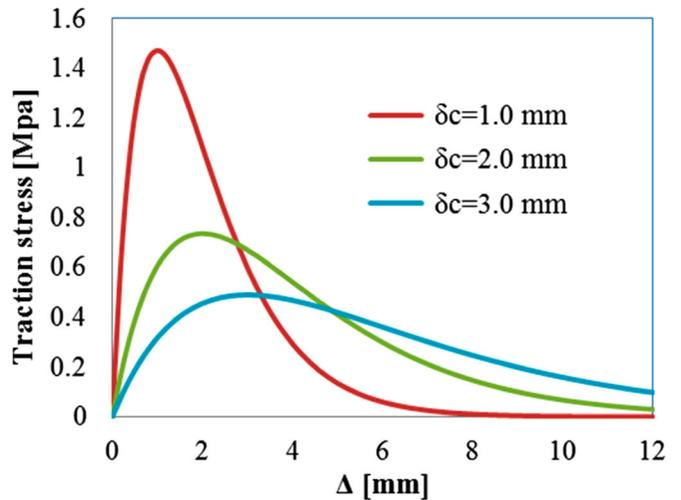
Figure 11. Traction-separation law ( $G = 4.0$  N/mm,  $\delta_c = 1.0\text{--}3.0$  mm).
