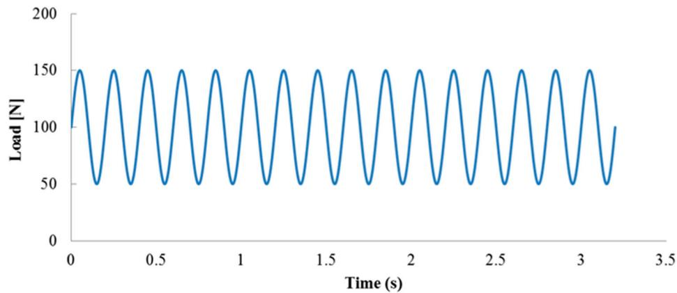
Figure 27. Load scheme of MAT cyclic tests.
