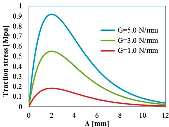
Figure 5. Traction-separation law ( $G = 1.0\text{--}5.0$  N/mm,  $\delta_c = 2.0$  mm).
