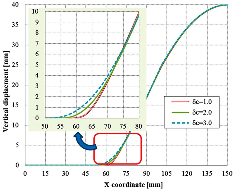
Figure 12. Membrane vertical displacements ( $G = 4.0$  N/mm,  $\delta_c = 1.0\text{--}3.0$  mm).
