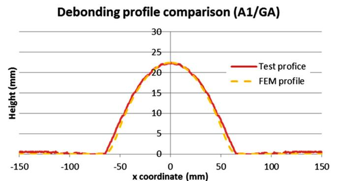
Figure 26. Debonding profile comparison between experimental and FEM results.
