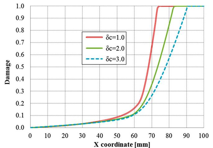
Figure 14. Interface damage ( $G = 4.0$  N/mm,  $\delta_c = 1.0\text{--}3.0$  mm).
