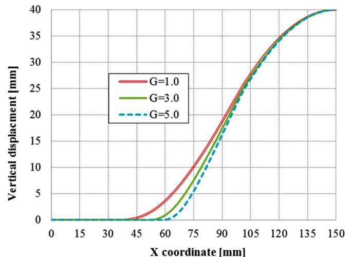
Figure 6. Membrane vertical displacements ( $G = 1.0\text{--}5.0$  N/mm,  $\delta_c = 2.0$  mm, displacement control load at piston is 40 mm).
