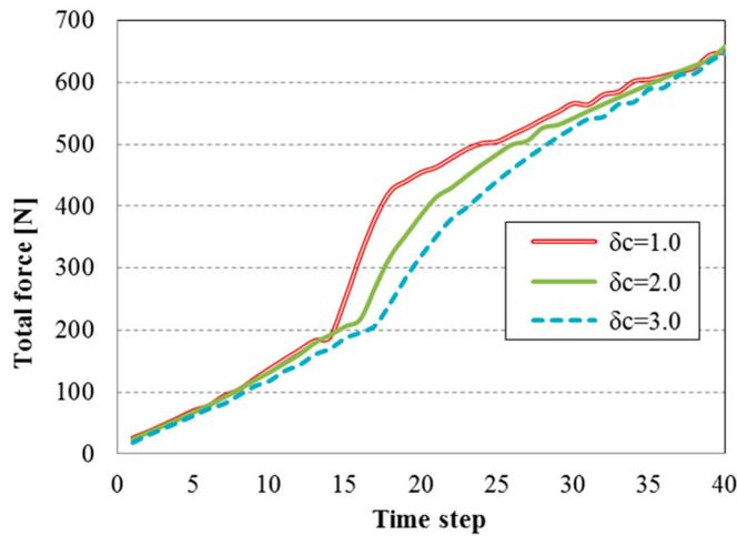
Figure 15. Piston total force ( $G = 4.0$  N/mm,  $\delta_c = 1.0$ – $3.0$  mm).
