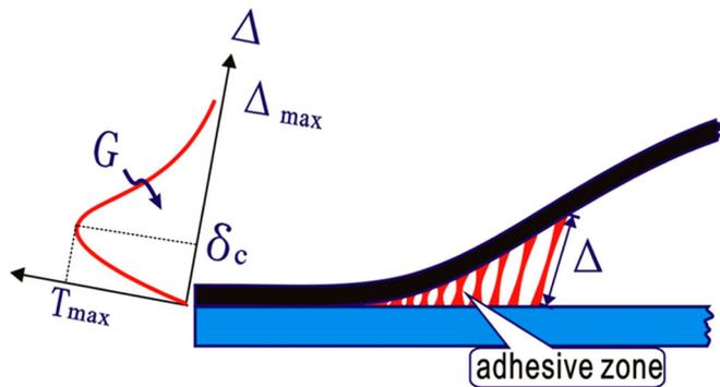
Figure 16. Schematic diagram of adhesive traction-separation model.
