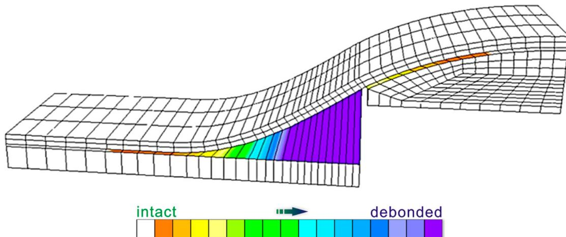
Figure 9. Interface damage distributions ( $G = 2.0$  N/mm,  $\delta_c = 2.0$  mm, displacement control load at piston is 40 mm).
