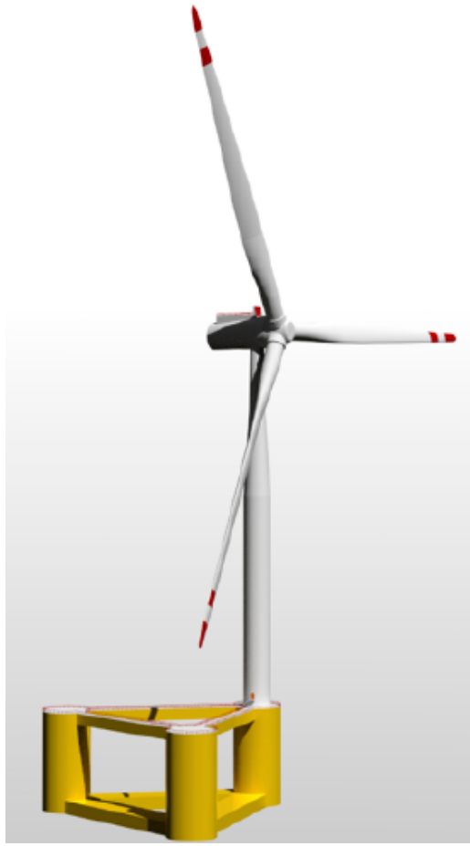
Figure 21: Visualization of the 12 MW WINDMOOR turbine on the INO-WINDMOOR semi-submersible (Figure 3.1, Inocean, Carlos Eduardo Silva de Souza et al. 2021)
