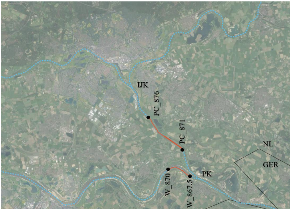
Figure B.5: Location for the dredging activities in the PC and the nourishments in the Waal. The labels indicate the river branch and the river kilometers according to the format 'riverbranch_rkm'.
