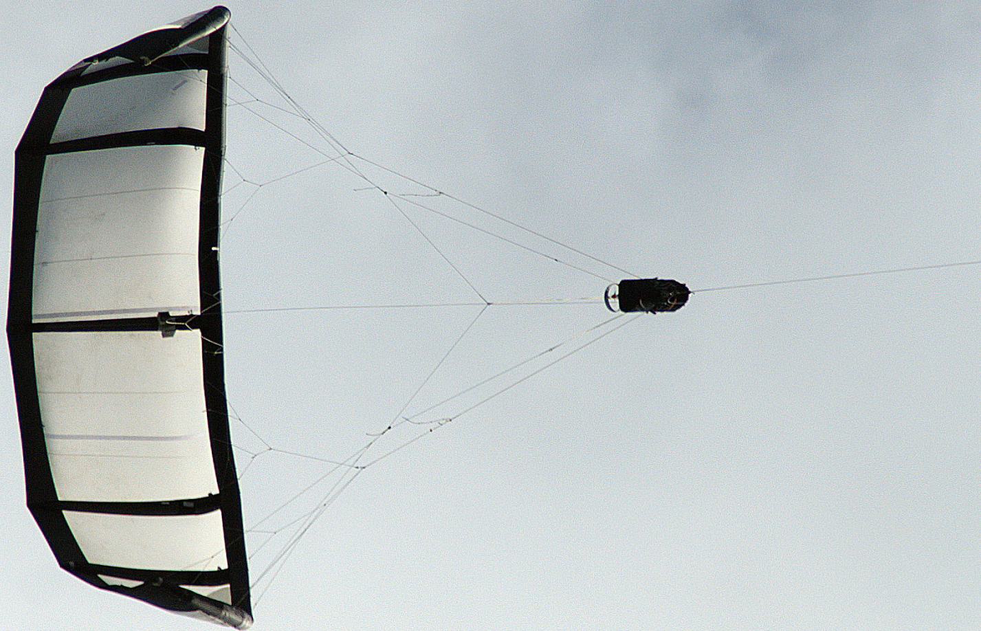
Kite Control Unit KCU2, designed and built by Kitepower and Maxon Motor, steering a 25 m 2 kite (24 July 2017)
