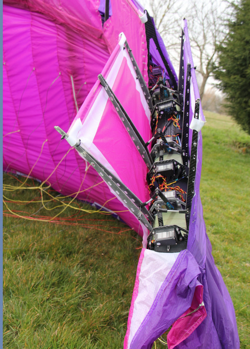
Aerodynamic control of the ram air wing of Kite Power Systems Ltd. (16 March 2015)
