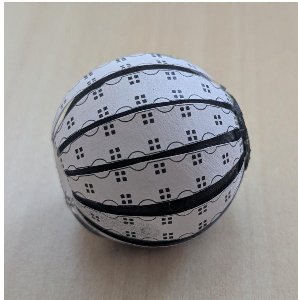
Figure 4.6: PCB printed on paper
