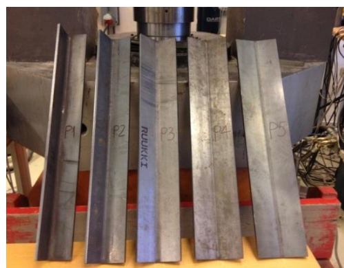
Fig. 1 L section profiles with different cold-formed angles
