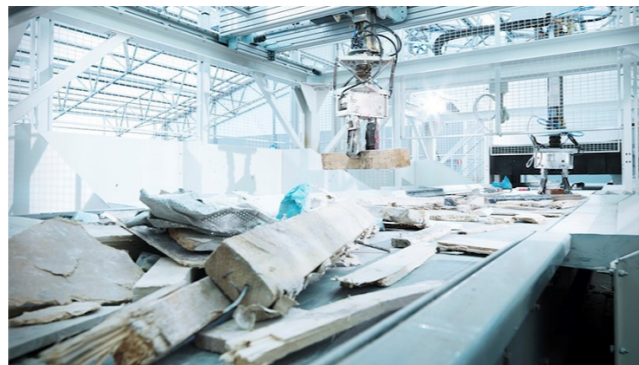
Figure 3.6 Robotic sorting of waste wood (recycling today)
