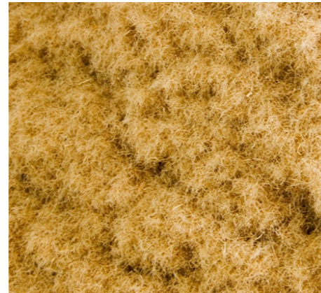
Figure Blown in wood fiber (isofloc)
