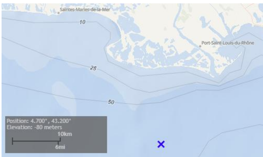
Figure 18: Location of offshore wave data with associated depth (NOAA Bathymetric data viewer)
