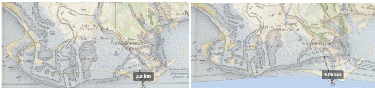
Figure 21: The georeferenced “Bouches du Rhône” map from 1827 overlaid on the current map of the Rhône delta. On the left the affine transformation is used while on the right the TPS transformation is used. The distance between the same point (the western bank of the mouth of the Grand-Rhône) on the 1827 and current map has been indicated for both types of transformations (Old Maps Online).
