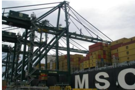
Figure 21: Super post panamax quay cranes at MSC Terminal in Valencia. Source: MSCTV (2010)
