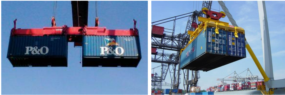
Figure 10 and 11 : A twin lift spreader (left) with a capacity of two 20 ft. containers and a tandem lift (right) with a capacity of two 40 ft. containers. Source: Port Strategy (2007 & 2009).
