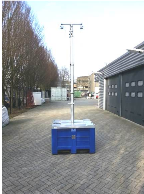
Figure 3.2: Multi-camera Stand Alone Video Installation (McSAVI)
