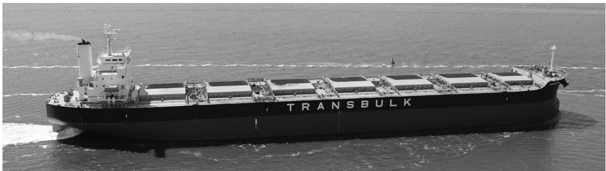
Figure B.3: A Panamax bulk ship; Yarrowonga (dwt: 82 [kt], L_s : 229 [m], B: 32 [m] and D: 14.6 [m]) (Courtesy of P. Jakobsen @Marinetrtraffic.com)
