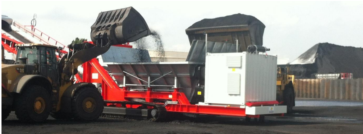
Figure 6.2: Handling of dry bulk materials using wheel loaders and a mobile feeding bunker (Courtesy of N.M. Heilig BV)
