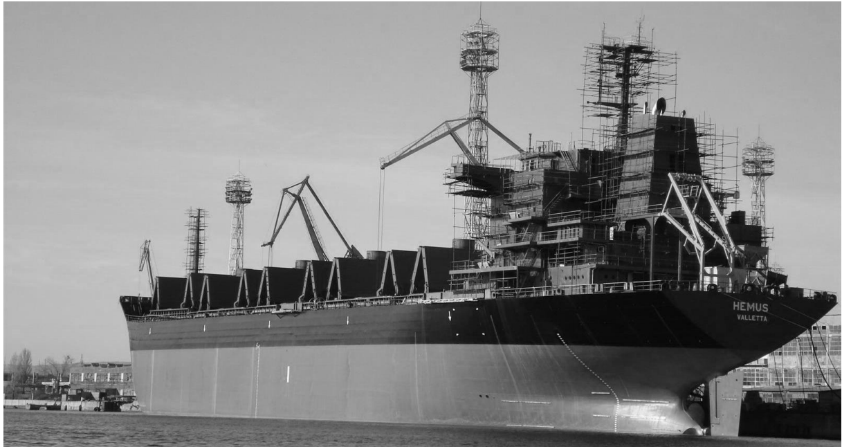
Figure B.2: An Handymax bulk ship; Hemus (dwt: 43 [kt], L_s : 186 [m], B: 30 [m] and D: 11.7 [m]) (Courtesy of Marinetrtraffic.com)
