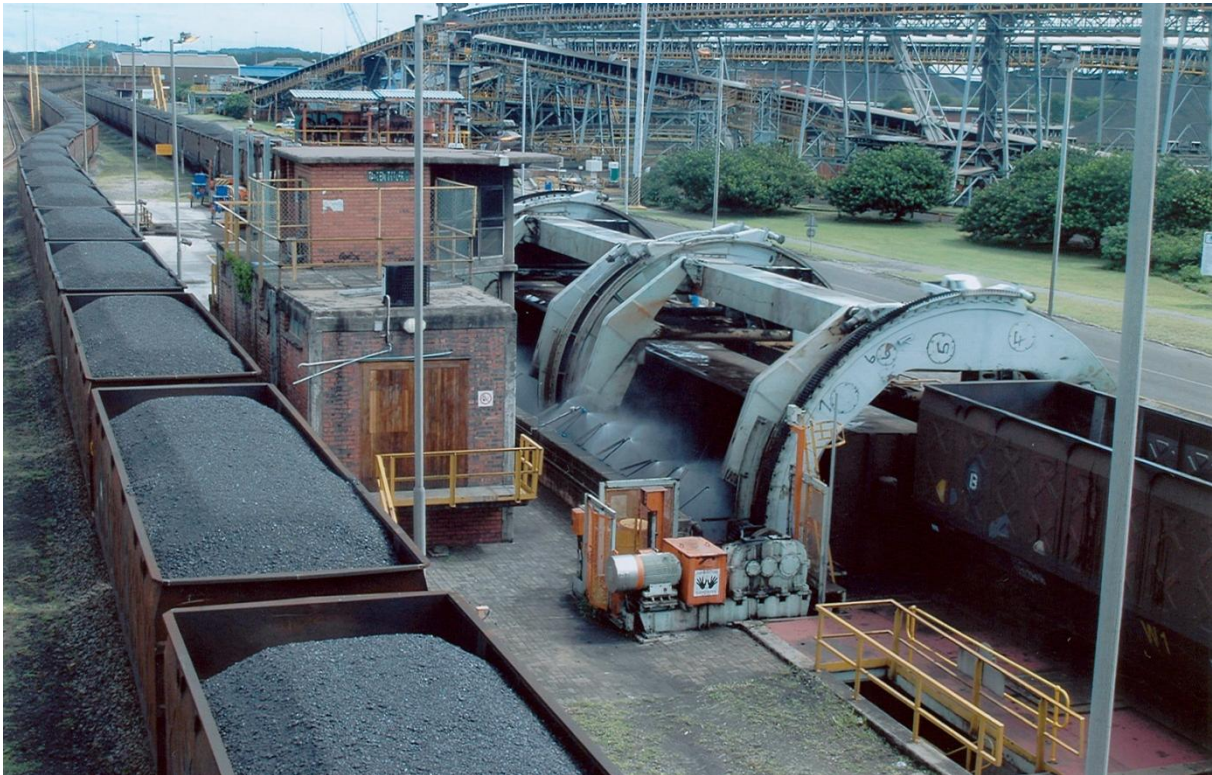
Figure 4.5: Rail cars unloading at the Richards Bay coal terminal (Courtesy of RBCT)
