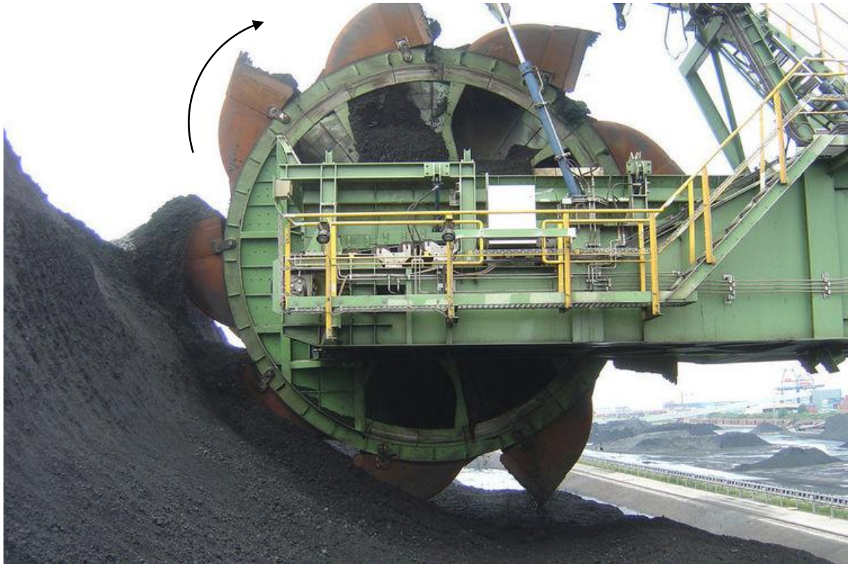
Figure 6.7: A bucket wheel reclaims material from a pile (Courtesy ThyssenKrupp)
