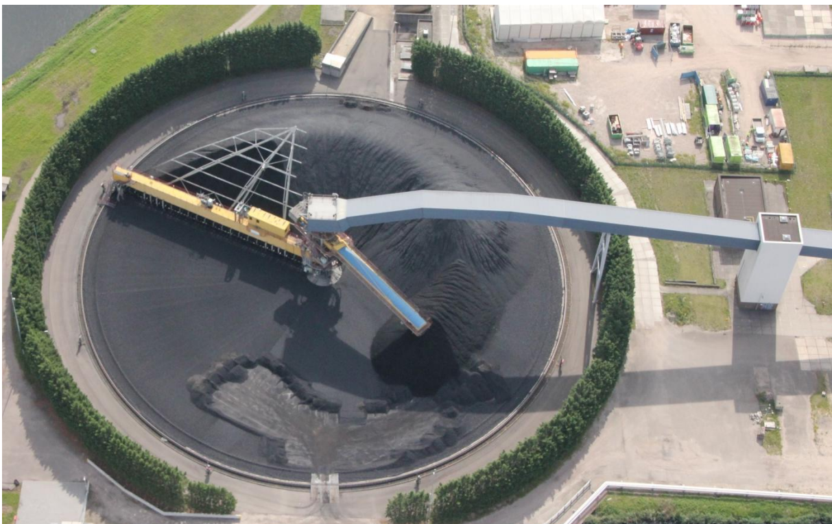
Figure 6.4: A circular storage system with a radial stacker and a bridge scraper reclaimer installed near a coal-fired power plant in Amsterdam (Courtesy Kees Vlot)
