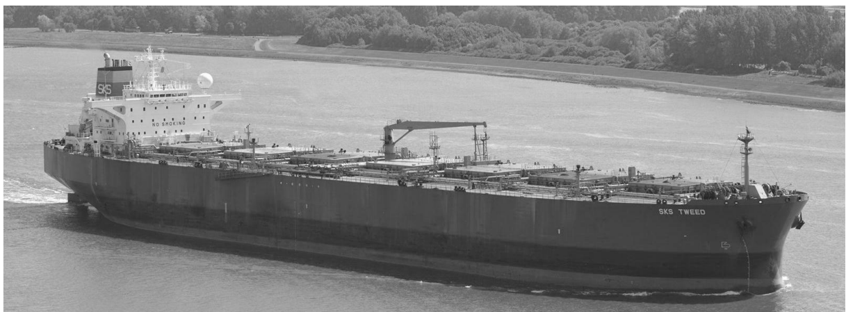
Figure B.4: A small Capesize bulk ship; SKS-Tweed (dwt: 110 [kt], L_s : 243 [m], B: 42 [m] and D: 15.7 [m]) (Courtesy R.Maats @Marinetrtraffic.com)
