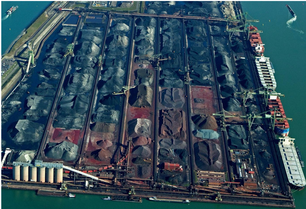
Figure 5.1: A stockyard with lanes and segregated piles (Courtesy of EMO BV)
