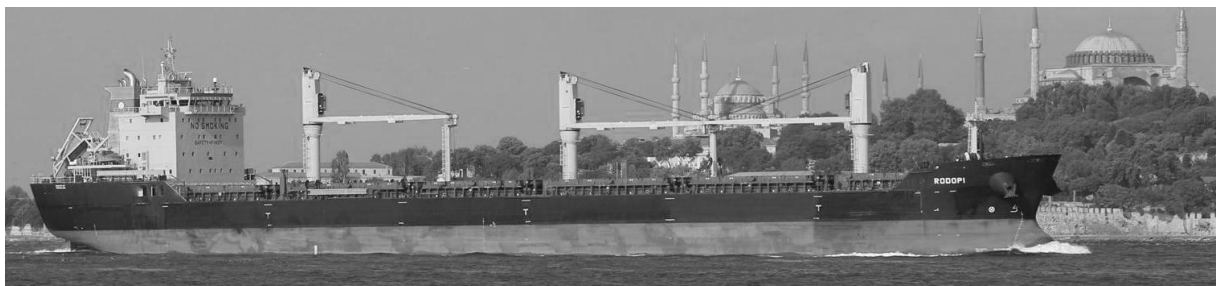
Figure B.1: An Handysize bulk ship; Rodopi (dwt: 23 [kt], L_s : 181 [m], B: 23 [m] and D: 10.4 [m]) (Courtesy of M. Guney @Marinetraffic.com)
