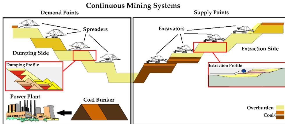
Figure 4. A schematic view of continuous mining systems, reproduced after (Gärtner, Hempel, & Rosenberg, 2013).
