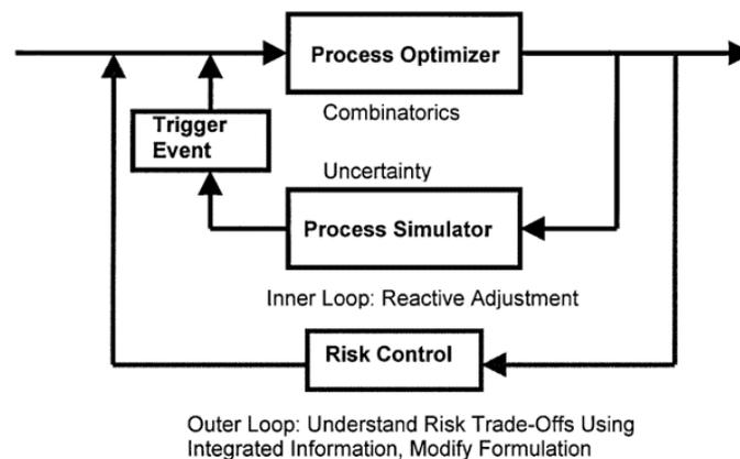
Figure 2. The “Sim-Opt” architecture (Subramanian et al., 2001).
