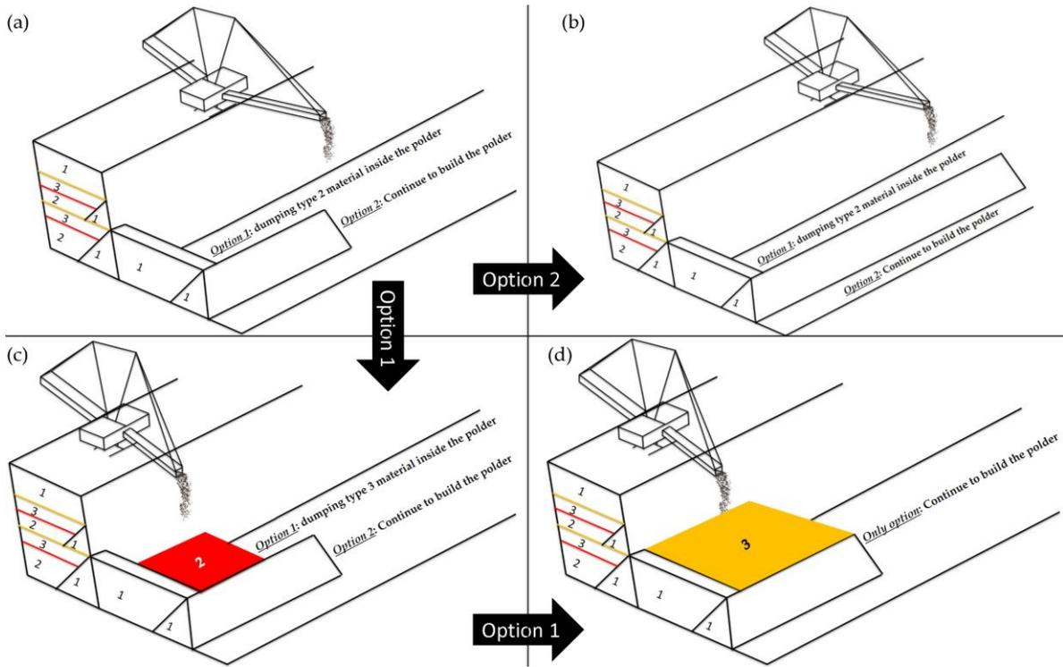
Figure 7. Schematic representations of dumping options.
