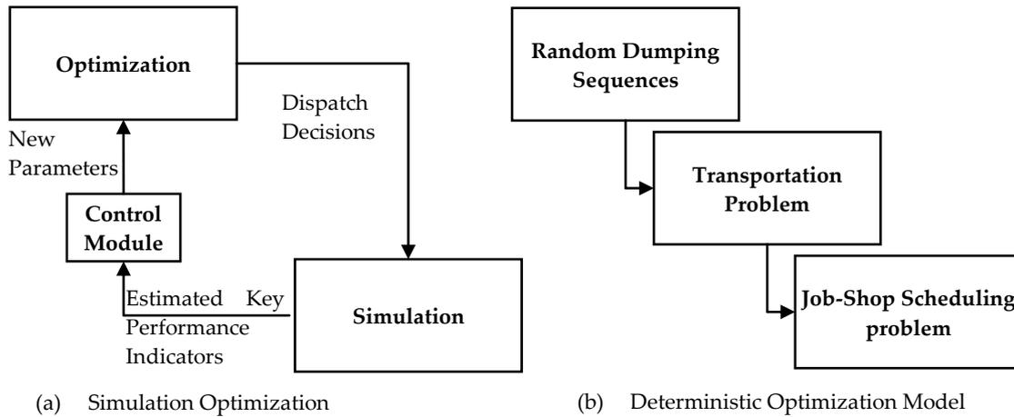
Figure 6. Configuration of the simulation-based optimization approach.
