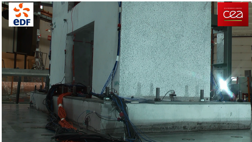
Figure 4.5: Foundation of the mock-up.
