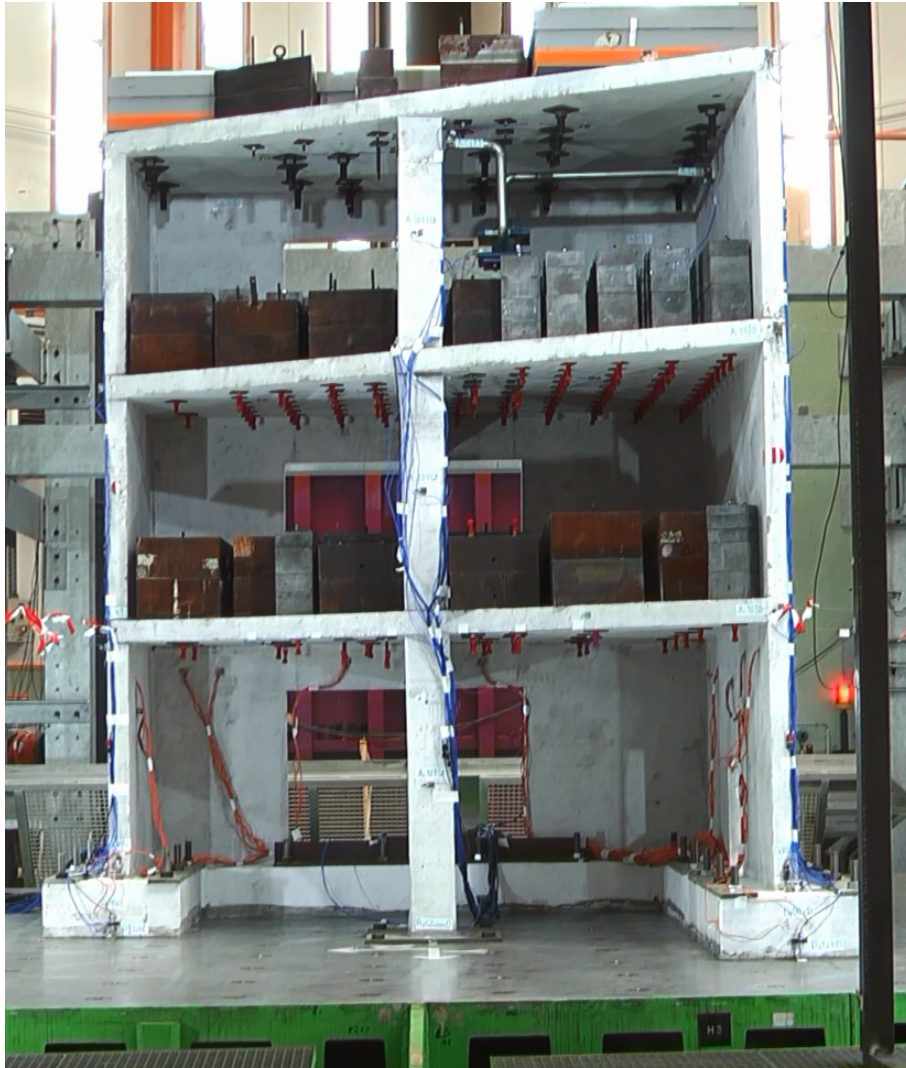
Figure 4.6: Reinforced concrete mock-up and additional masses.
