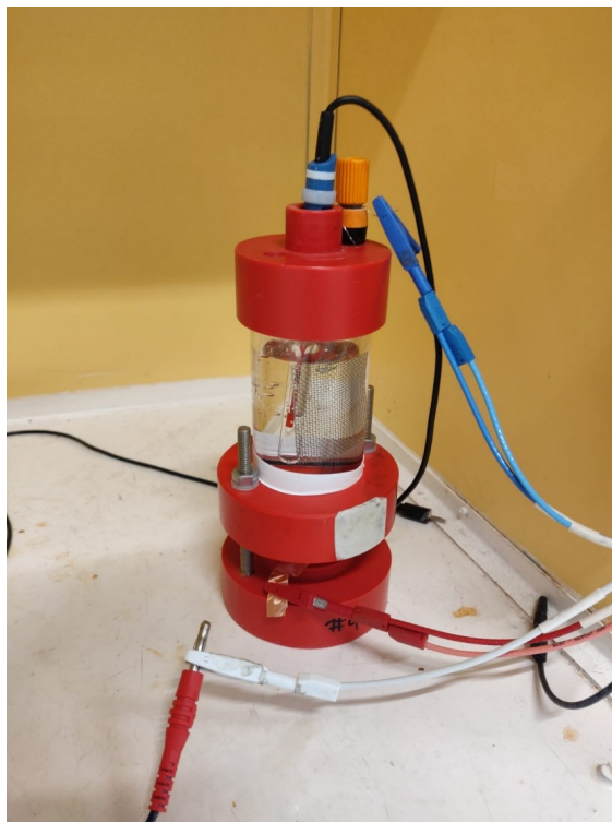
Figure 25: Setup of the electrochemical cell, in which the red wire is connected to the working electrode via the copper tape, the white wire is connected to the SCE reference electrode and the blue wire is connected to the stainless steel counter electrode. The solution consists of 3.5 gram NaCl solved in 100 mL distilled water, and the exposed surface area is a circle with a 1 mm diameter.
