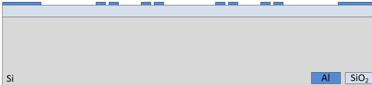
Figure 4.2: The first steps of the MEMS actuator fabrication: Sacrificial layer deposition and Al heater definition by sputtering and wet etching.
