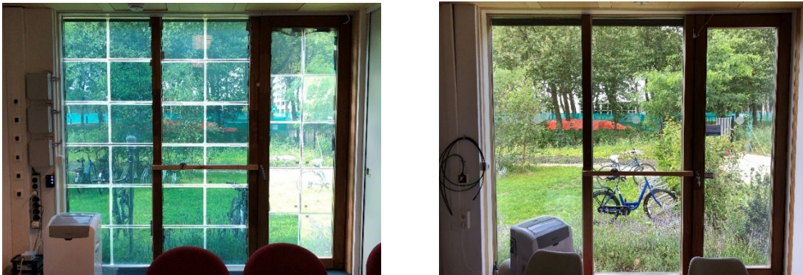
Figure 1. West façade of the experimental room with EC triple glass IGUs (left) and of the control room with standard triple glass IGUs (right). In the operable window, six of the small panes faced material leakage issues resulting from the lamination process due to improper sealing and could not be used.
