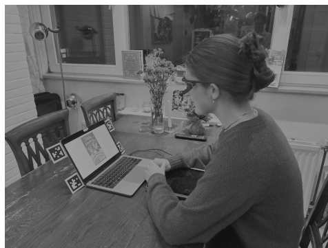
Figure 5.8: Photograph of eye tracking experimental set up with posing participant.
