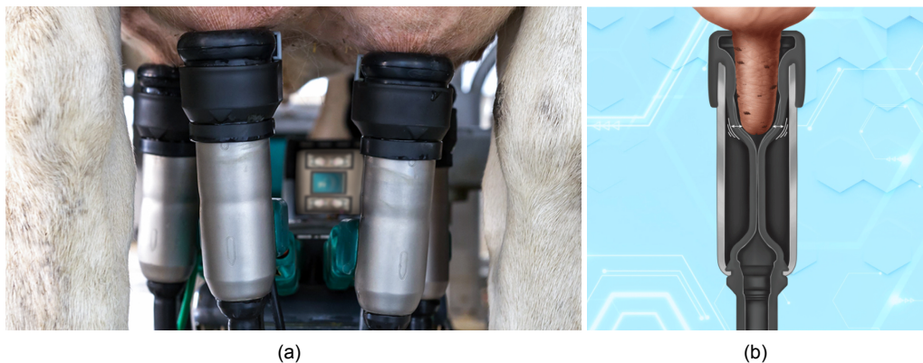
Figure 1.4: (a) The GEA DairyRobot R9500 executes the pretreatment and milking process in the same teat cup (b) stimulation of the teat is done by vibrating the liner inside the cup, similar to the milking technique but with less power [6].
