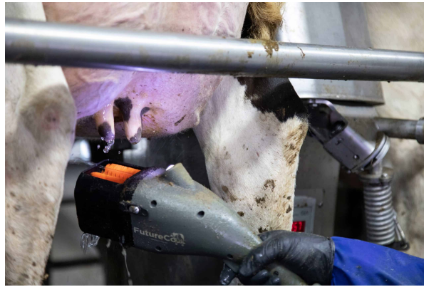
Figure 4.5: The FutureCow Teatscrubber is used to clean and stimulate the cow's teats after forestripping [28].
