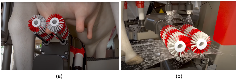
Figure 4.1: (a) The two counter rotating brushes of the Lely Astronaut A5 clean and stimulate the teat (b) the brushes get disinfected after the pretreatment [40].
