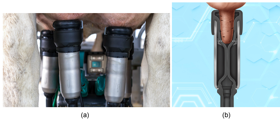
Figure 4.3: (a) The GEA DairyRobot R9500 executes the pretreatment and milking process in the same teat cup (b) stimulation of the teat is done by vibrating the liner inside the cup, similar to the milking technique but with less power [30].
