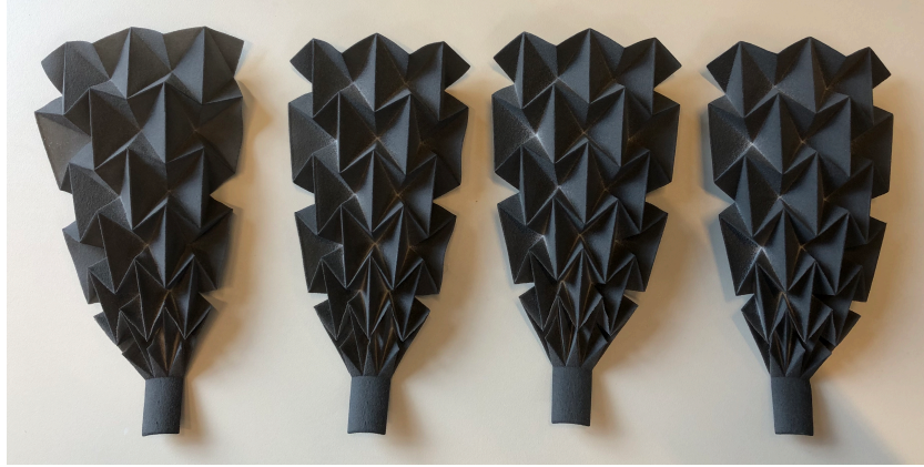
Figure G.2: Four 3D test-prints to see what wall thickness still has acceptable quality, ranging from 0.2 mm to 0.8 mm, left to right
