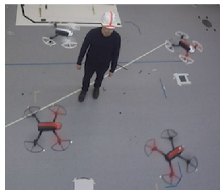
Fig. 1 Four drones in a square formation avoid a walking human
