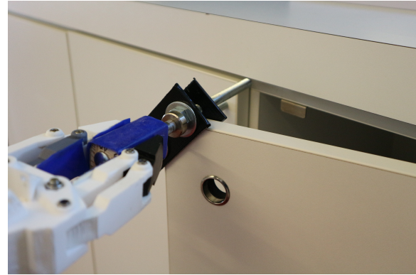
Figure 3-4: The magnetic tool can be grabbed by the robot.
