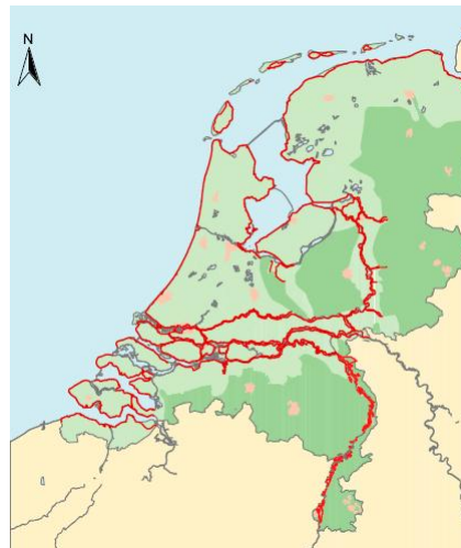
Figure 1.1.: Areas in the Netherlands threatened by sea and river (light-green). Higher grounds are indicated with a dark-green colour. The primary water defense is indicated in red. ( HR2006, 2007 )
