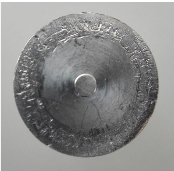
Figure B2 - Impression of the surface of the joint containing wear of the surface due to locking of the rods.
