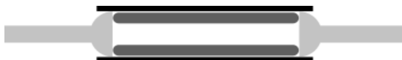
Figure 3.1 – 2D impression of the basic components of the mechanism. Black elements represent the frame, dark grey represent the transmission, light grey represent the joints.
