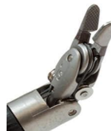
Figure 1.2 - Cable driven steerable instrument Endowrist developed by Intuitive Surgical [6]. Image adopted from Intuitive Surgical
