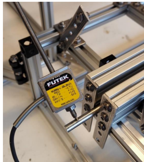
Figure E.3 - Impression of the covidien instrument tested in the setup (above), left a close-up of the force sensor touching the tip. Right shows the reference measurement in which the compliancy of the setup was evaluated. In this case the angled setup.
