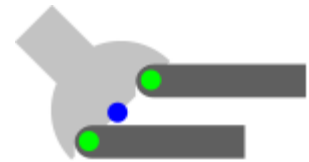
Figure 3.6 - Rods no longer enclosed by the hole if the steering angle is equal of larger than 45 degree.
