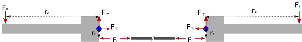
Figure 2.1 - Force analysis of steering mechanism. Dark grey element represent the transmission and in light grey the joints. The blue point indicates the rotation point of the joint.
