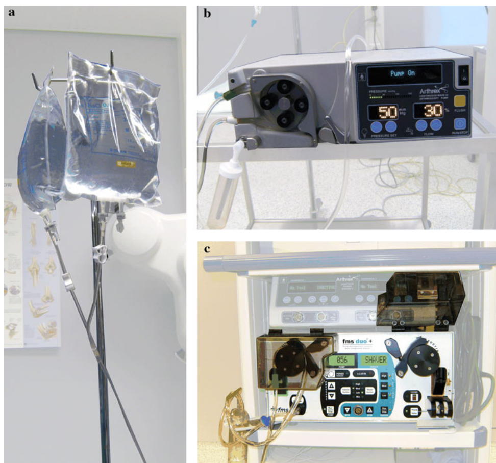
Fig. 1 Three arthroscopic irrigation systems were assessed for their performance with automated blood detection: a gravity infusion, b single roller pump, and c double roller pump. For the gravity
