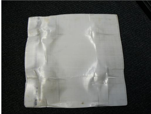
**Figure 1.10:** *Delamination in Dyneema composite due to impact*
