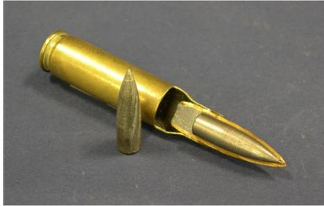
**Figure 2.10:** *non-deformable 7.62 AP munition. Courtesy of TNO.*
