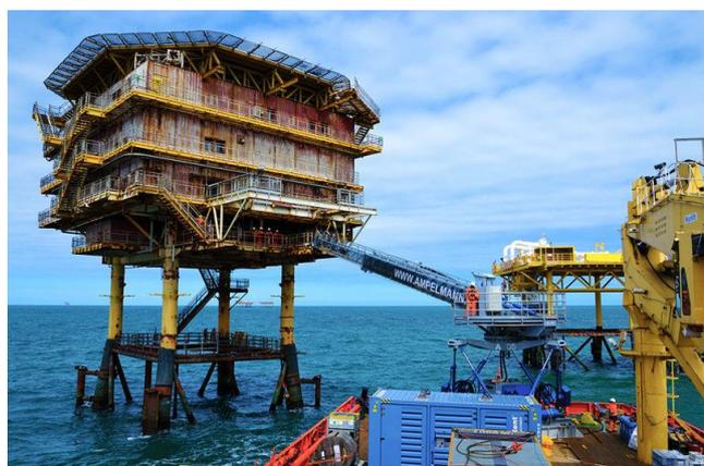
Figure 1-2 An Ampelmann system connected to a fixed offshore platform.
