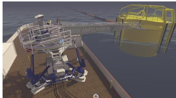
Figure 1-3 Visual representation of a connected Ampelmann system to a CALM buoy.
