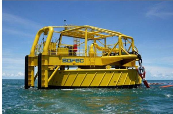
Figure 2-4 SOFEC CALM buoy.
