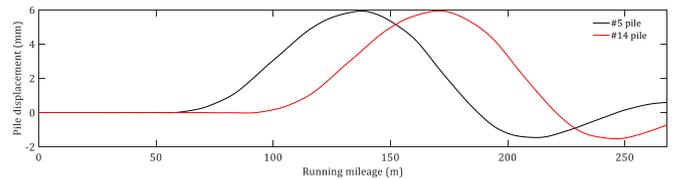
Fig. 13. Vertical displacement of piles #5 and #14.
