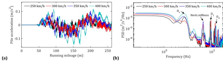
Fig. 20. Comparison of pile acceleration at observation point #5 (a. time history; b. PSD curve).
