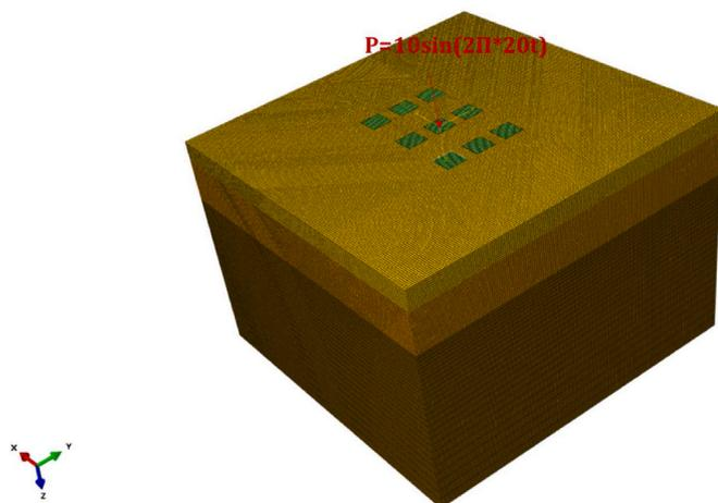
Fig. 9. Pile-soil interaction model established in ABAQUS.
