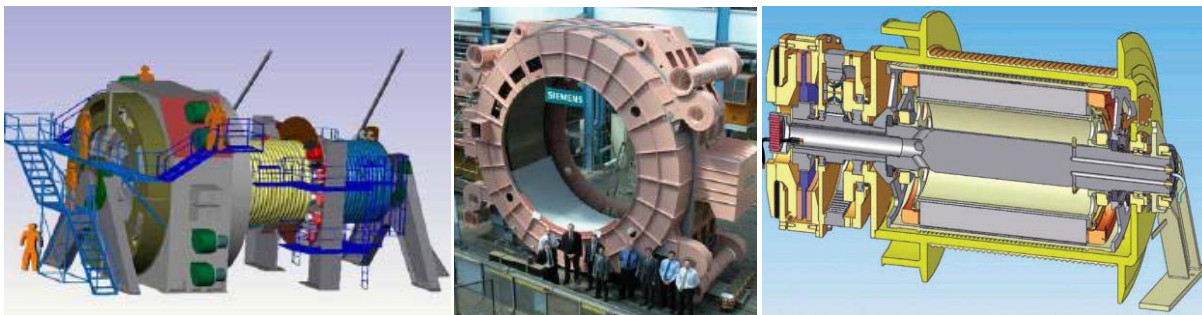
Figure 8.7 (left and center): AC synchronous motor installed in a walking dragline
