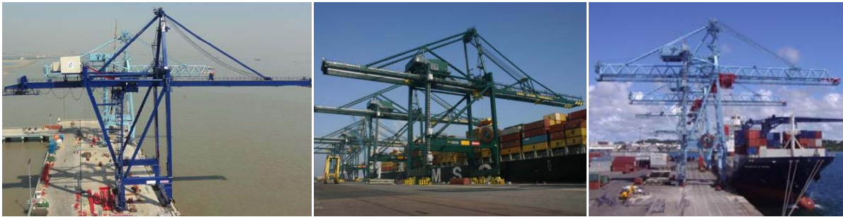
Figure 1.4: Three types of STS crane girders: (from left to right): Monobox girder, Double box girder and lattice girder
