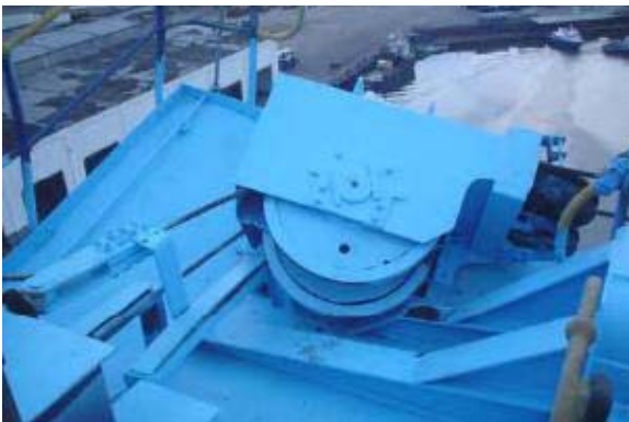
Figure 1.8: Example of damage caused by snag: plastic deformation of rope sheave mounting at the tip of the boom. Extreme rope tension caused by snag bent the sheaves upwards [4]
