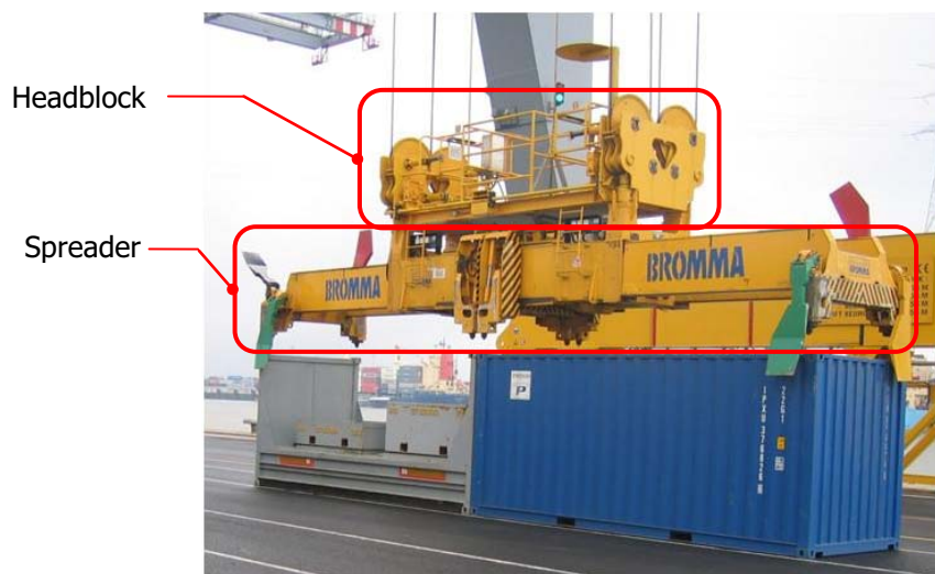
Figure 1.5: Headblock and spreader in twinlift mode, with an open top and a standard 20' container. All 8 container corners will be connected using twistlocks on the spreader (source: Cargotec)
