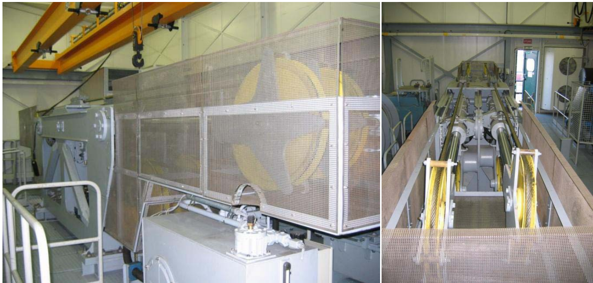
Figure B.4: picture of the anti-snag device installed in an STS-crane at the MSC Delwaidedok terminal in Antwerp (source: Cargotec)
