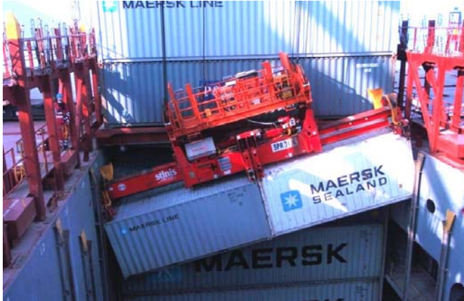
Figure 1.6 (left): Example of a snagged load caused by skewing in the ship cell, in this case two 20'-containers on a twin-lift spreader (Source: Cargotec)
