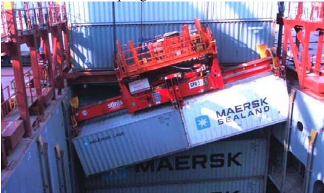
Fig 1: Example of a snag due to skewing of the container (source: Cargotec)
