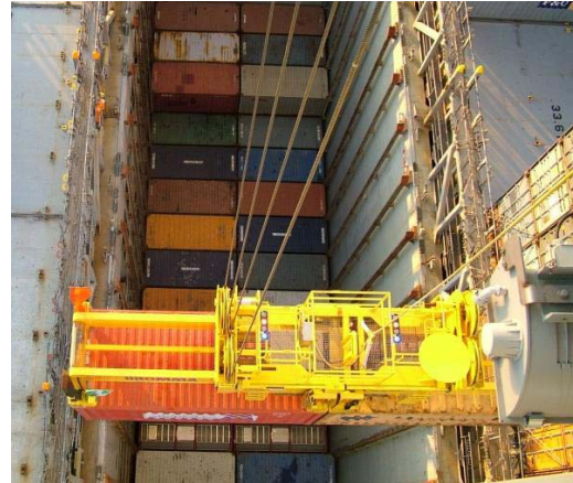
Figure 1.6 (left): Example of a snagged load caused by skewing in the ship cell, in this case two 20'-containers on a twin-lift spreader (Source: Cargotec)
