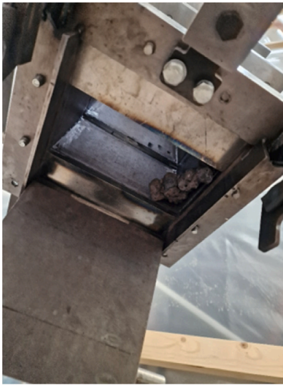
Fig. 17. Photograph taken at the end of a sinter charging experiment, showing accumulated sinter particles at the hopper outlet.
