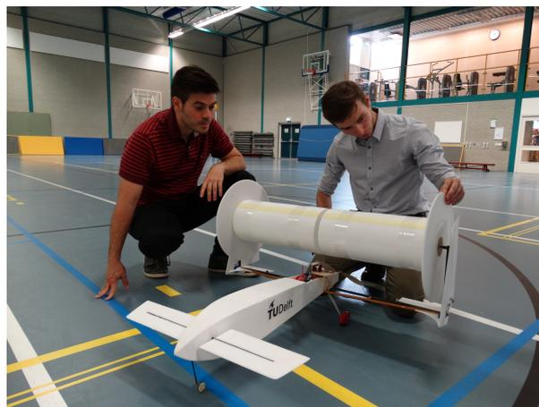
Figure 5.20: RC Model after the addition of endplates
