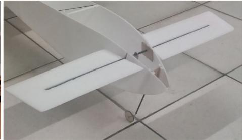
Figure 5.17: Canard with carbon spar and nose gear installment
