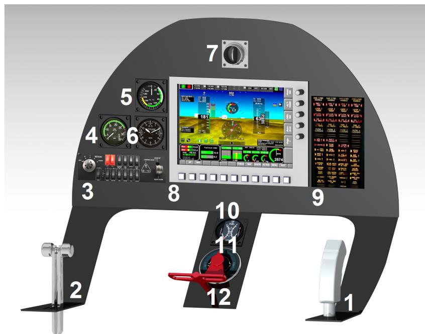
Figure 3.50: Cockpit control panel, with instruments indicated as: 1) Sidestick, 2)Throttle ICE, 3) Landing Gear switch + starter panel, 4) Backup cylinder rpm indicator, 5) Backup speed indicator, 6) Backup altitude indicator, 7) Ventilation, 8) Integrated EFIS, 9) Warning/failure panel, 10) Fuel tank indicator, 11) Fuel indicator, 12) Ballistic Recovery System trigger
