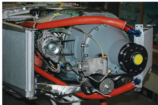
Figure 3.46: Example of the radiator attachment [34]
