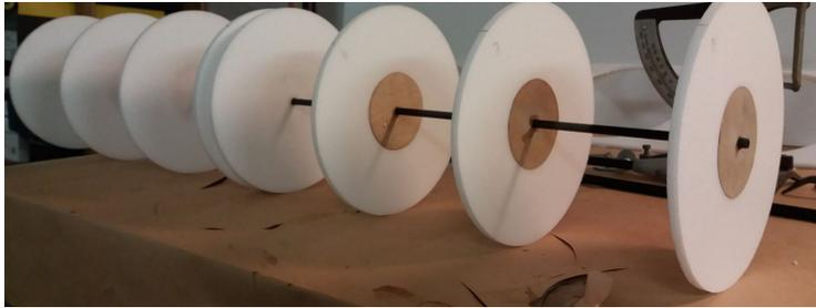
Figure 5.16: Structure of cylinder with carbon spar and noma plan ribs, reinforced with multiplex
