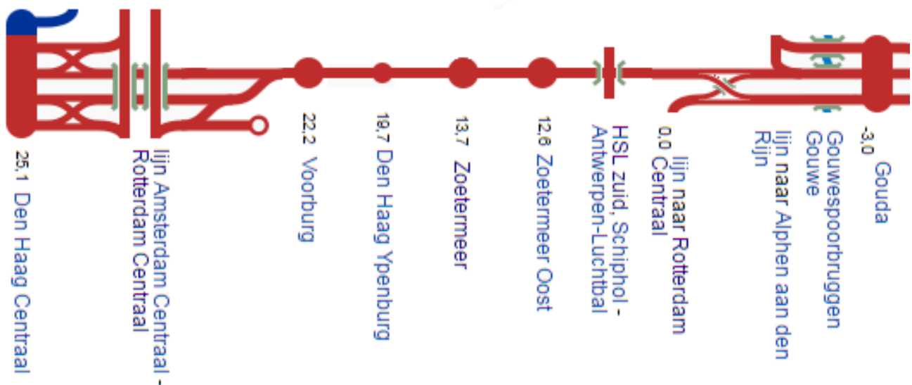
Figure 2.21: Layout of railway line Den Haag Centraal - Gouda. With all stations and mileage
