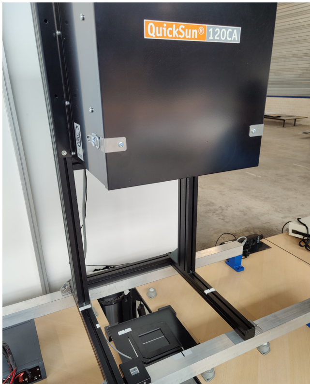
figure A, setup of IV measurements
