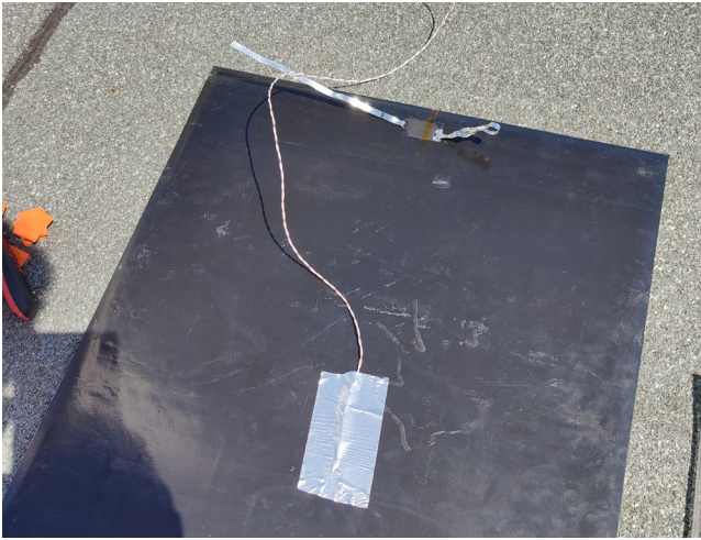
Figure A, first layer of heat conducting tape to transfer heat to temperature probe.
