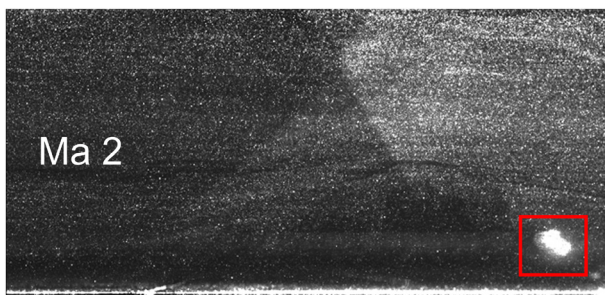
FIG. 5. Instantaneous particle image of SWBLI (Mach 2.0, Mach reflection).
