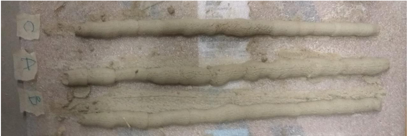
Fig. 4.14 Open time specimens
