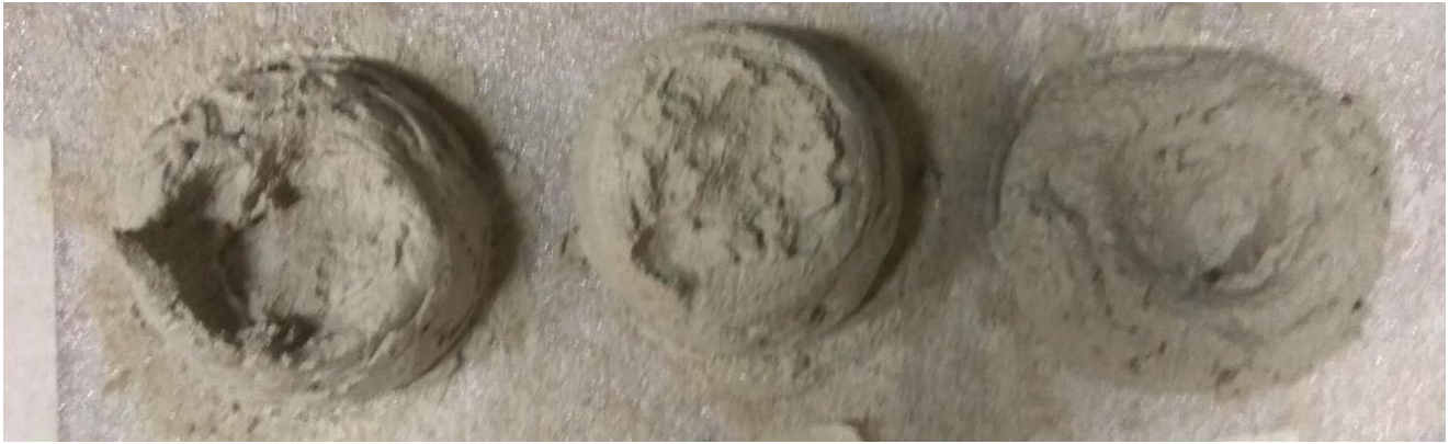
Fig. 4.13 Flowability test cone samples
