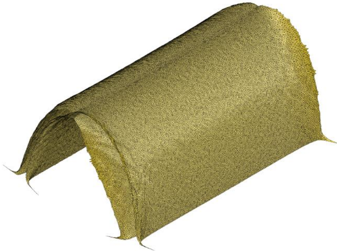
Fig. 9.6 Karamba3D Resulting vault mesh
