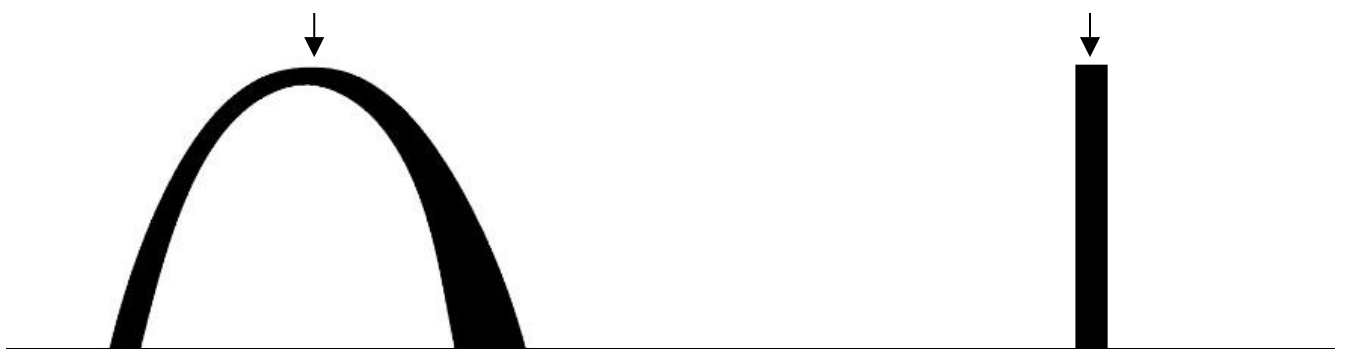
Fig. 5.19 Buckling analysis approximation
